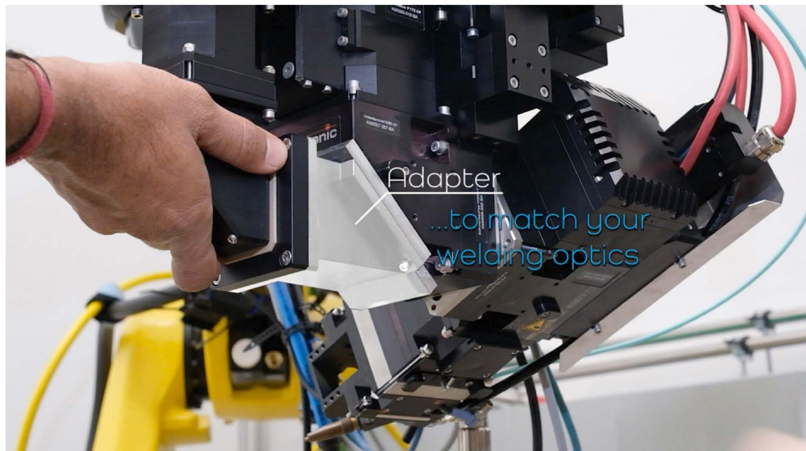
Fig. 1 The video (online version of this article) shows how the OCT SCANNER is mounted to the ALO processing head
