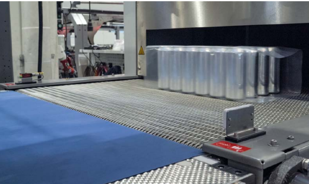
Conveyor belt transition upstream of the shrink tunnel. The blue textile conveyor belt is deflected with Iglidur P210 knife edge rollers which are continuously subjected to temperatures of up to 100 °C.
