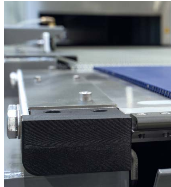
Iglidur knife edge rollers can be used not only with PU and textile belts, but also with modular belts.
