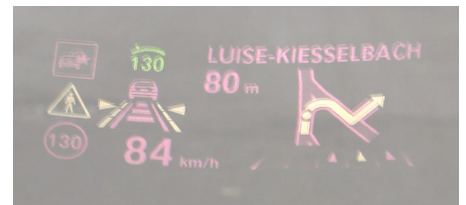
Distortion of an HUD projection caused by misalignment of the optical path within the HUD engine.
