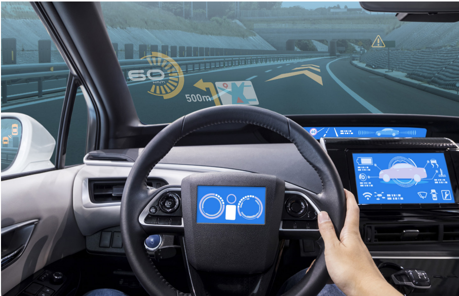
Figure 1 - As with AR displays, HUD projections must be visible at precise locations projected onto an infinite plane. Ensuring correct position, color, brightness, and clarity of HUD images augments the operator experience and limits error that may cause distraction.
