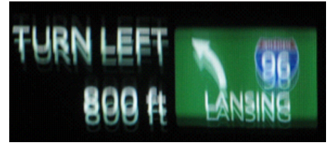
Ghosting of the image is caused by misalignment of HUD projections that are reflected back from the windshield.
