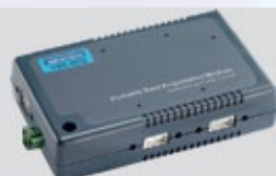
USB-4620 Isolierter 5-Port-Full-Speed- USB-2.0-Hub
