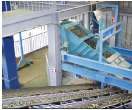
Fig. 4: Mogensen SC1026 and the three downstream belts with the various grain sizes
