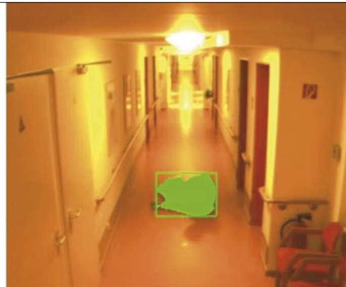
A person is detected as moving and is tracked automatically for further analysis (top), the movement is classified as fall (bottom)
