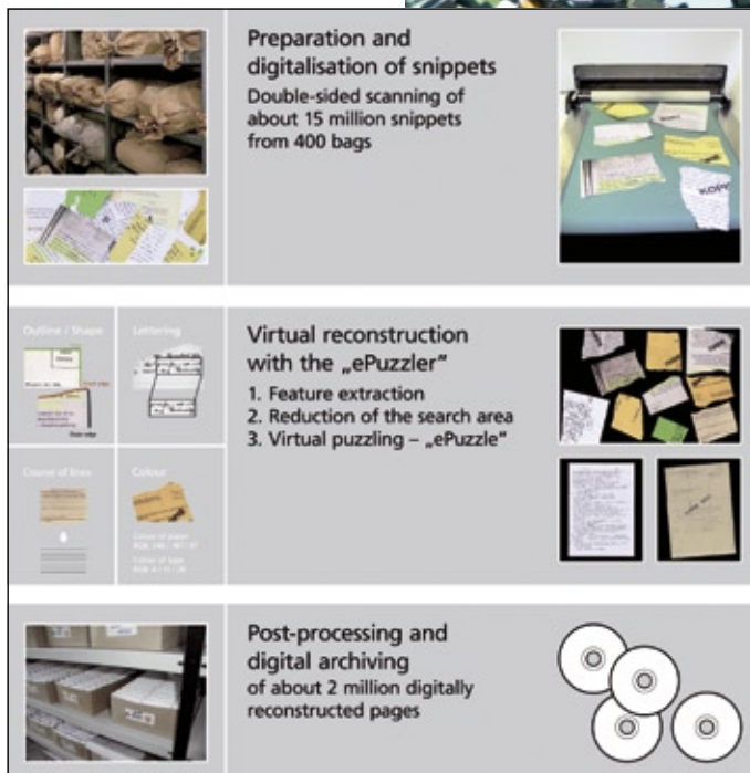
Fig. 1: Complete process. Before the reconstruction takes place, the snippets have to be digitised double-sided. The virtual reconstruction, consisting of three parallelized steps, takes place. As shown in the middle, different features of the snippets are extracted to find the right reconstruction partners. After a data transfer the snippets are processed and archived digitally.
