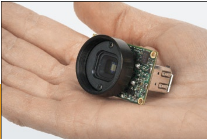
Tiny 29x40mm Firefly MV IEEE-1394 digital camera
