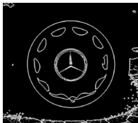
Fig. 3: a) original image; b) boundaries have been isolated and thinned; c) contrast-enhanced version of the accumulator after Hough-transform applied to the boundaries
