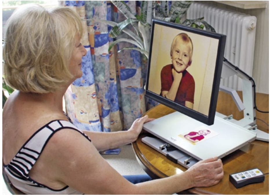
Screen reading aids fitted with high high-power camera modules assist the elderly in reading text and viewing image documents
