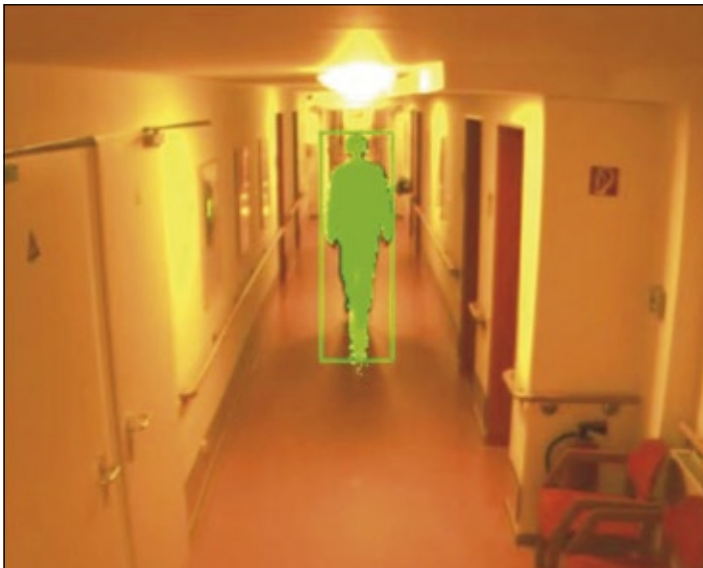
A person is detected as moving and is tracked automatically for further analysis (top), the movement is classified as fall (bottom)
