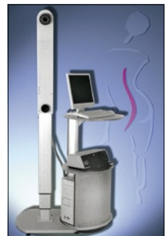
A complete 3D model of the spine is reproduced from the stereographic image of the back taken with a uEye camera from IDS
