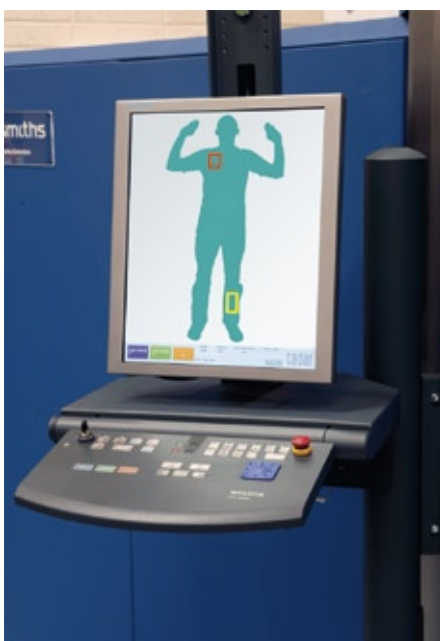
Smiths Detection's innovative millimetre-wave approach automatically detects concealed threat objects hidden under layers of clothing
