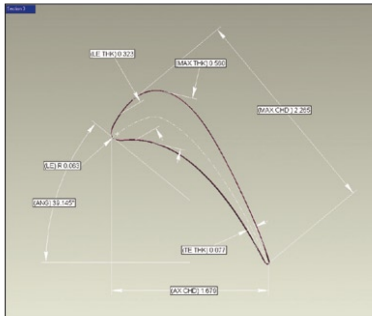
Fig. 5: 2D sectioning and dimensioning
