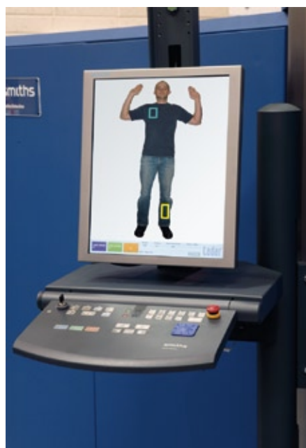
A privacy filter works with the automatic detection software to identify the concealed object without displaying body images
