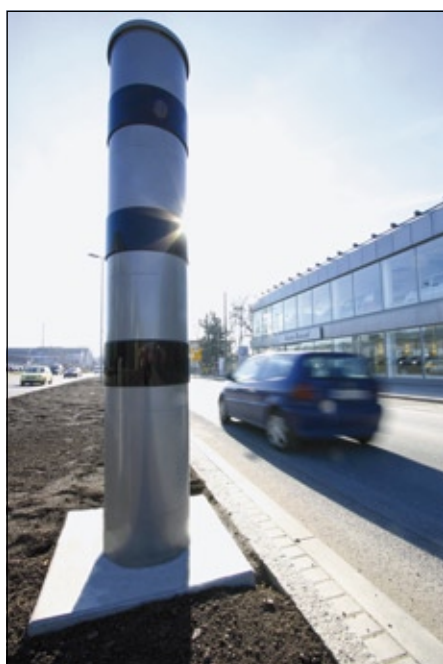
PoliScan speed system with a fixed city housing contains rotatable segments
