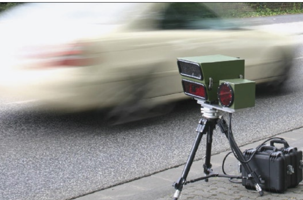
PoliScan speed can be quickly mounted on a tripod without the need for on-site calibration
