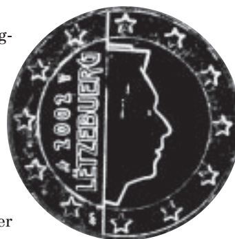
Fig. 1: Dark-field lighting of a coin enhances the edges on the surface
