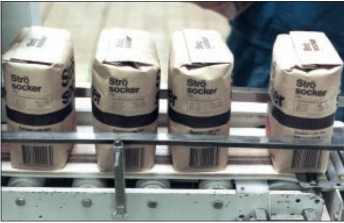
Every sugar bag coming out of the packaging machine needs to be inspected
