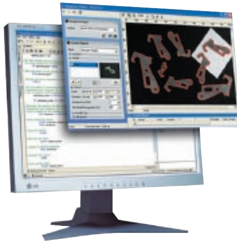
AdeptSight Vision uses a geometric object locator for part recognition
