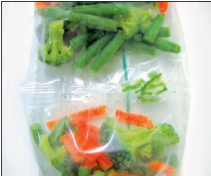
Food residue in the seal area causes major issues and makes this food package a complete waste product
