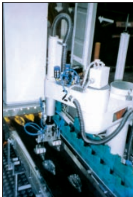
Vision guided Scara robot doing bottle sorting
