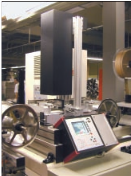
The integrated monitor and membrane keypad for programming the SAC VisionCube system directly are especially convenient
