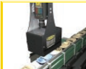
Car Door Handle Colour Inspection Colour detection of car interior door handles
