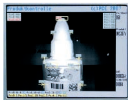
PCE Product control cameras analyze a maximum of 30 measuring windows simultaneously
