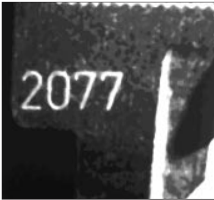
Fig. 2: Dark-field lighting of embossed numbers on a shiny surface
