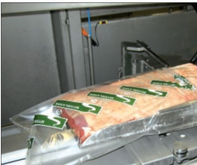
The bagging equipment presents the optimized packaging for the measured and identified meat cut
