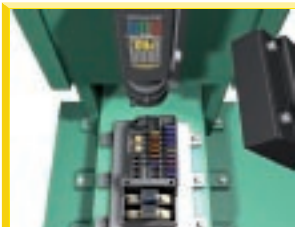
Automotive Fuse Box Inspection To verify that in a Fuse Box, rated fuses are correctly located
