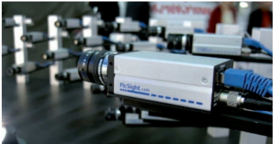
The intelligent Leutron Vision PicSight Smart cameras offer OEM users the choice of 28 image sensor types and an integrated Gigabit Ethernet port
