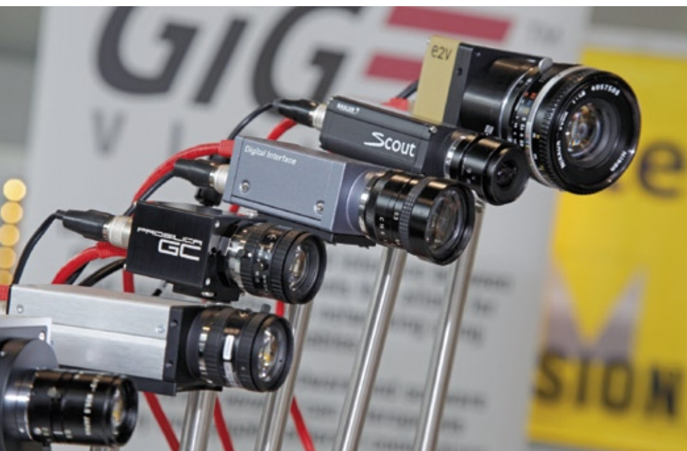
Any GenICam compliant camera can be easily connected as this demonstrator showed at Vision 2009 in Stuttgart
