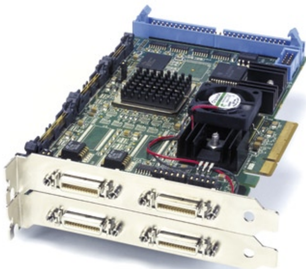
Configurable frame grabbers can support four base or two full and 10-tap Camera Link cameras as shown with BitFlow's Karbon CL-4 (Photo by BitFlow, Inc.)
