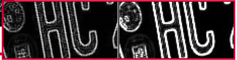
Fig. 2: Grey level image, dilated grey level image (upper part) and the difference of these images (lower left part); in the right left part the result of a Sobel filter for comparison, with enlarged detail from the edge images
