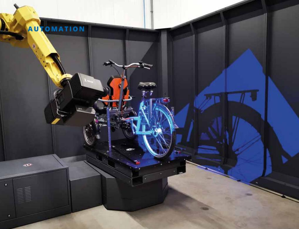
The full-area scans enable the bicycle manufacturer to inspect 100 percent of the manufactured components and then respond with targeted corrective measures.
