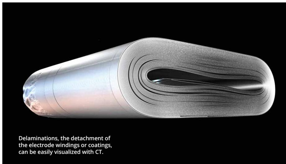
Delaminations, the detachment of the electrode windings or coatings, can be easily visualized with CT.
