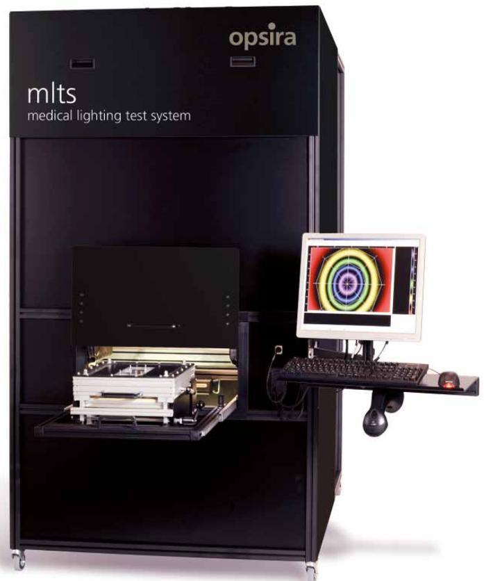
Based on a photometrically corrected measuring camera, the MLTS medical luminaire test stand from Opsira enables fast and high-resolution measurement and testing of illuminance distributions.
