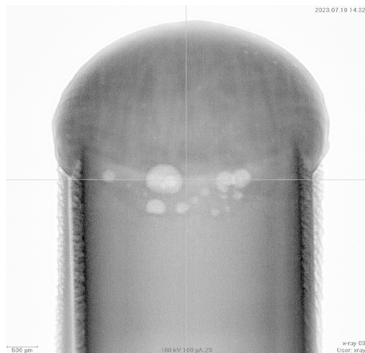
The higher rotation speed of the bifocal optics significantly reduces the frequency of pores in the upper part of the weld seam
