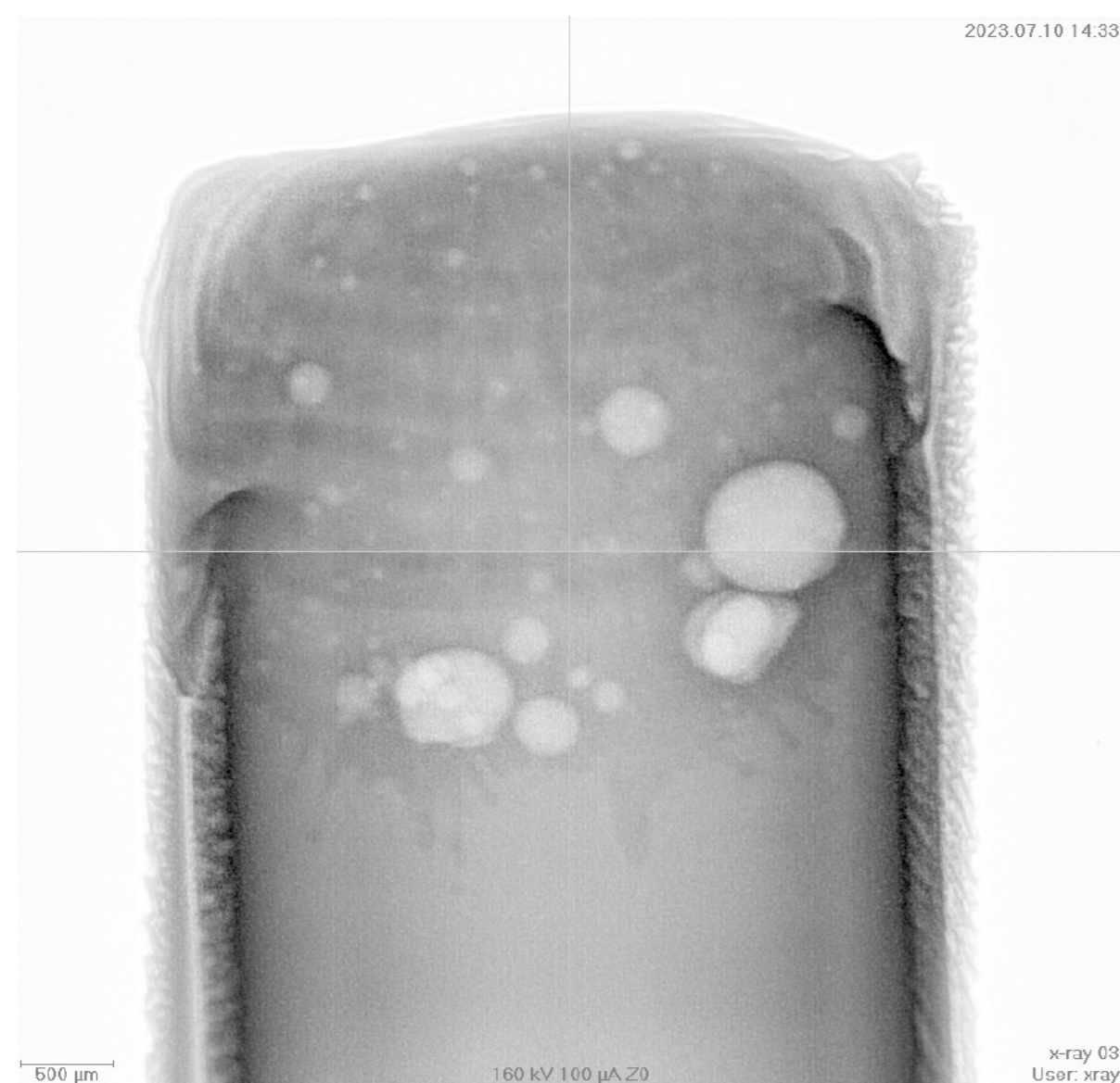
The higher rotation speed of the bifocal optics significantly reduces the frequency of pores in the upper part of the weld seam
