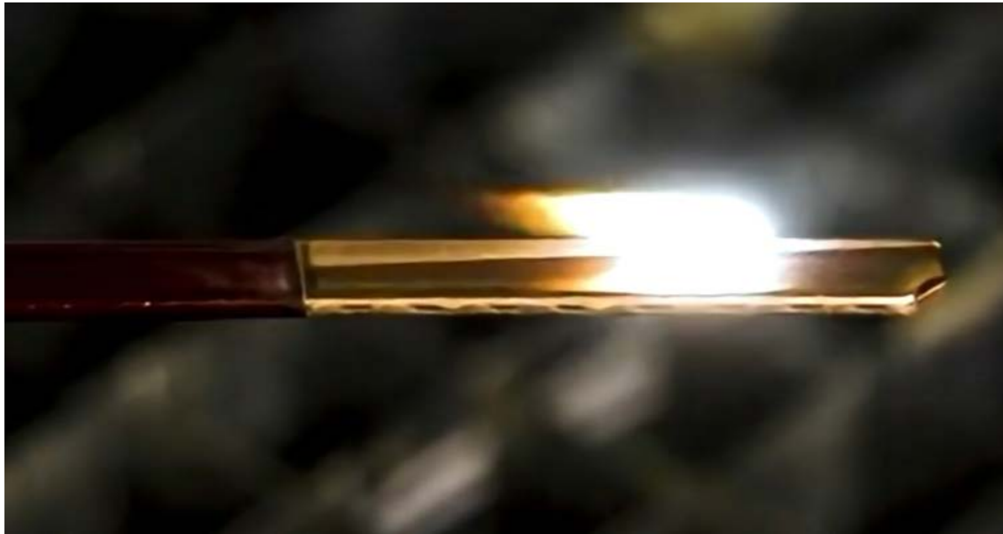
Fig. 5 Ablation of a hairpin with a Luxinar CO 2 laser. For a video, please see the e-special version of the article at https://indd.adobe.com
