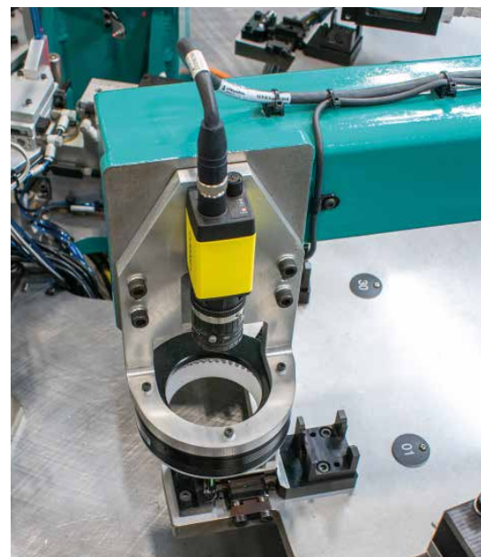
For ignition coil quality testing, SDC implemented several smart cameras from the In-Sight 8000 family.
