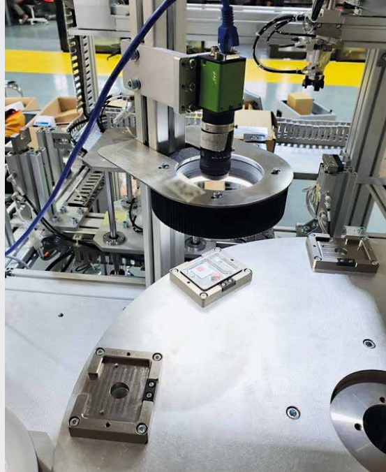
34 Cameras Ensure Perfectly Placed Heat Sinks
