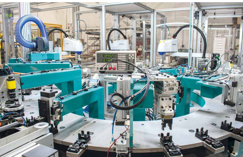
Customized factory automation systems from SDC and machine vision from Cognex ensure effective quality inspection of automotive ignition coils.
