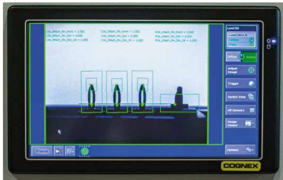
Cognex touchscreen displays show plant personnel failures that occur in real time, enabling faster optimization of production processes.
