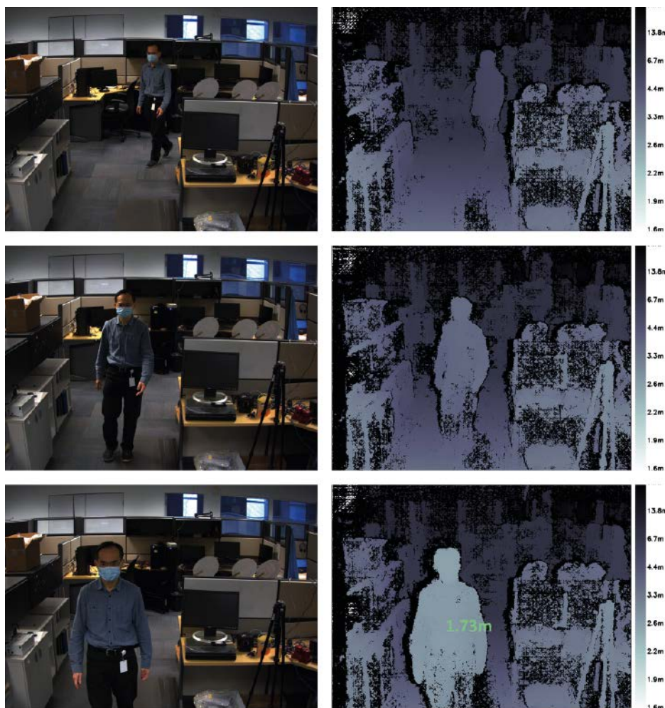
Figure 3: Sample left camera images and corresponding depth map. The bottom depth map also shows the depth at a particular point.
