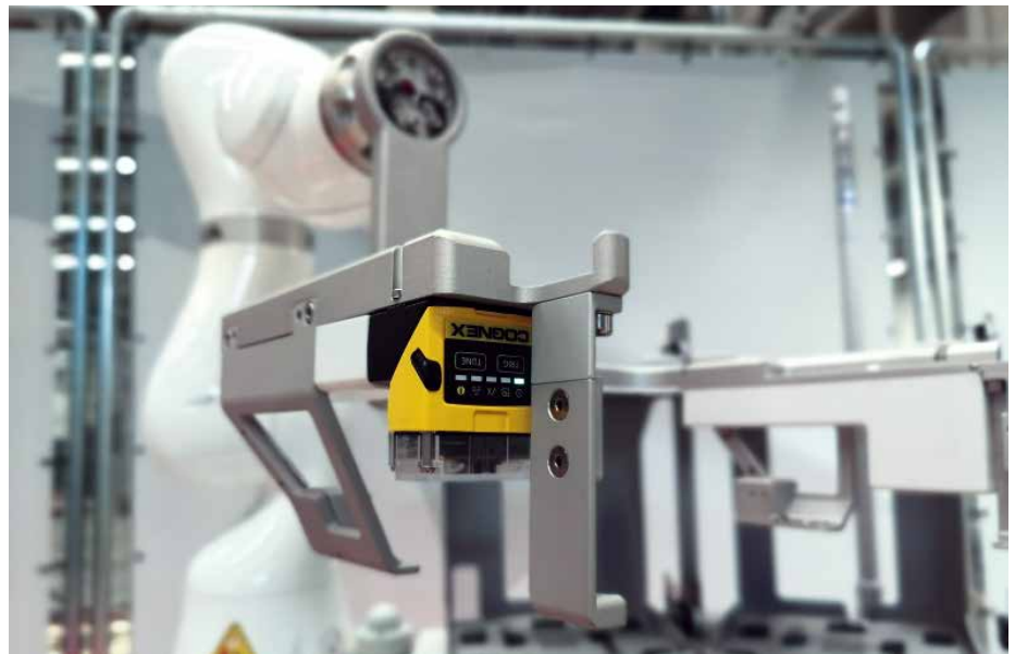
The gripping process itself is guided by image processing.
