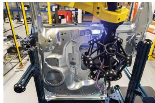
A robot-mounted optical CMM scanner during quality control of a car door
