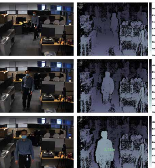
Figure 3: Sample left camera images and corresponding depth map. The bottom depth map also shows the depth at a particular point.
