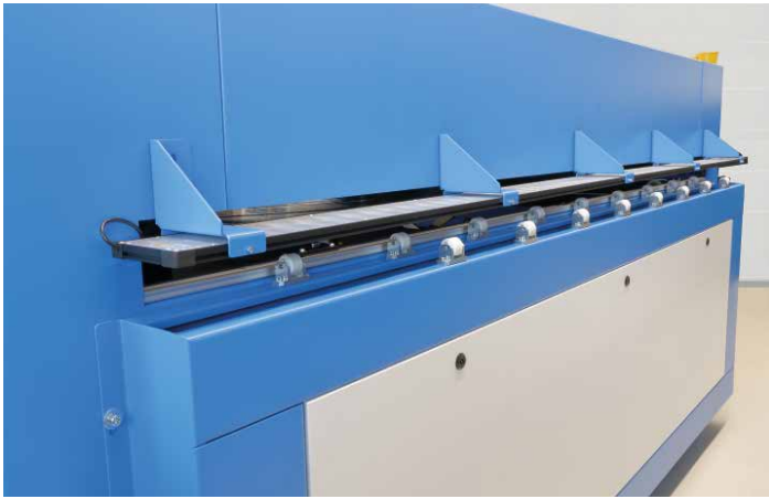
The 2.5 m long illumination from the MBJ Imaging Flex series mounted onto the Solar Module EL-quickline inspection system. The solar modules are measured in motion, during loading. Inside the machine, another inspection takes place: electroluminescence imaging.
