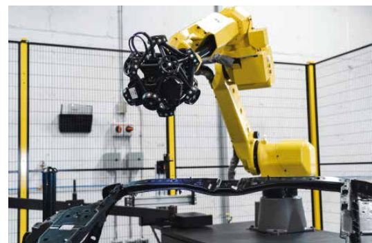
Robot-guided optical CMM scanner during quality control of a chassis.
