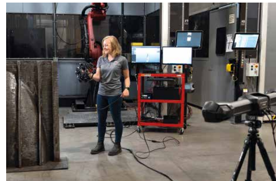
Lincoln Electric Additive Solutions chose 3D measurement technology from Creaform – more specifically, the Metrascan 3D – to create 3D surface models of its 3D-printed metal parts and compare them to the original CAD.
