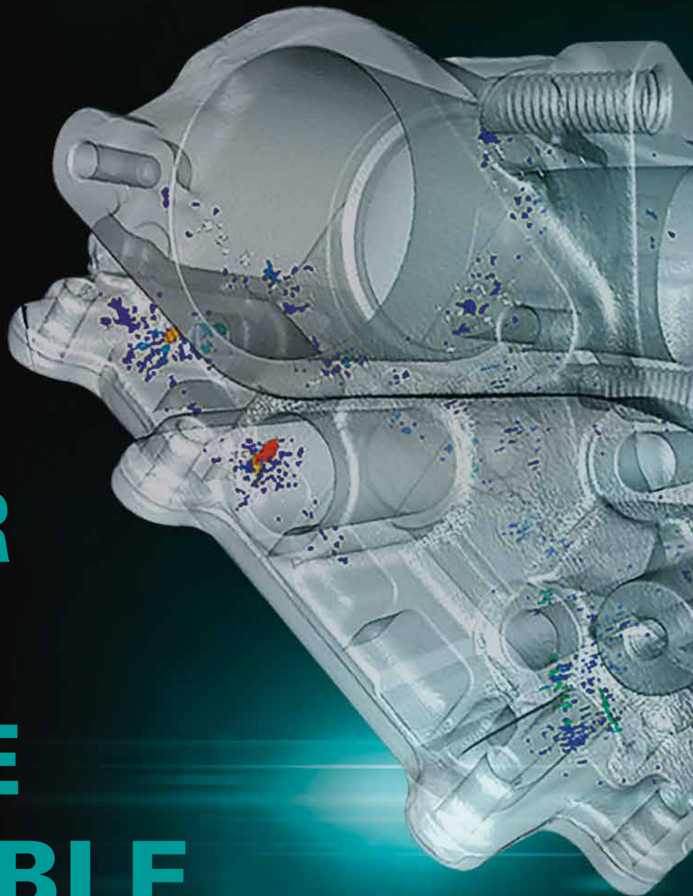
CT volume of a cast part with porosity analysis scanned by YXLON UX20
