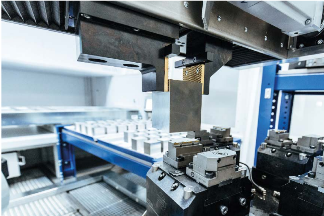
A KR Quantec from Kuka takes over the loading and unloading of the components automatically with a gripper from the Zimmer Group.
