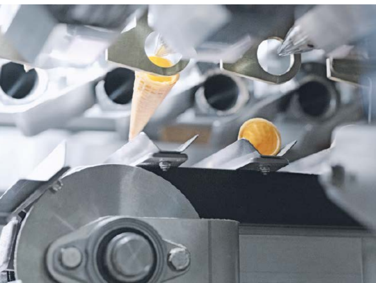
The shaping process for a typical wafer – an ice cream cone for example: The dough is poured on to individual baking plates (illustrated), which circulate through the oven at up to 0.5 m/s. At the end of the process the wafer is shaped into a pointed cone.
