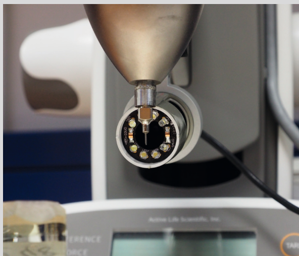
Figure 2: Medical nano-indenter for analysis of mechanical properties of bone used by the team of Dr. Busse
