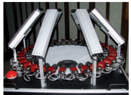
This exhibition demo illustrates the principle of a daisy chain network with direct FireWire connection from camera to camera
