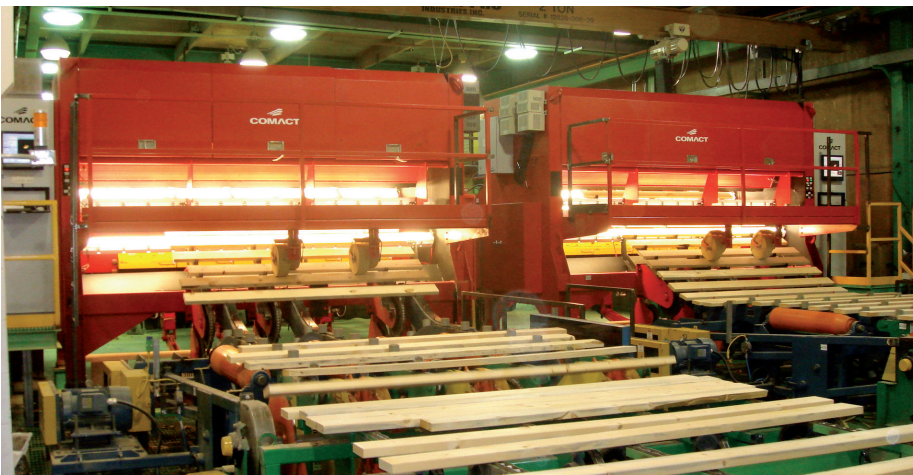
Fig. 3: This sawmill uses machine vision to determine where a rough-cut board will be divided into standard lengths in order to eliminate defects while maximizing the length of the resulting lumber (Image courtesy of Comact)
