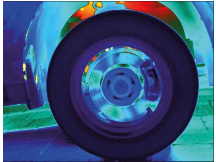
Brake rotor testing using high speed thermal camera at 60 fps
