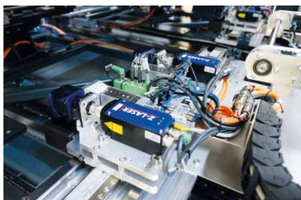
In the P2 structuring machine, two laser processing heads are operated in parallel, which is why two Z-Laser illumination lasers are used on one unit.
