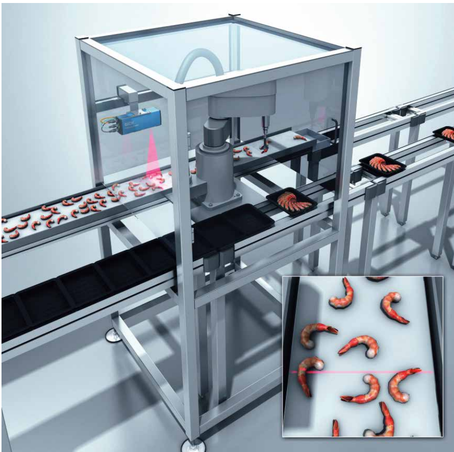
Vision systems guide the robots to pick the products from the automated conveyor line and place them into the desired packages. This ensures a consistent output quality both in primary packaging of food products, as well as in secondary packaging.
