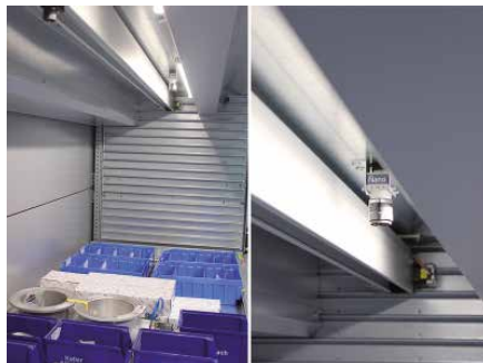
Fig. 4 Two Genie Nano cameras from Teledyne Dalsa, each with a fish-eye lens from Goyo, are used in each tower.
