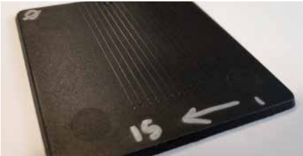
Fig. 1: Sample plaques can be used to test the effect of additives on scratch resistance.
