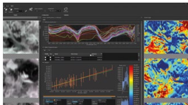
Fig. 2: Quantitative measurement of the net calorific value (NCV) of the bulk material: on the left: HSI input images in a spectrally averaged and standardised intensity; in the centre/top: sets of reference spectra as well as feature curve for the measurement of the net calorific value (green), table showing the measuring values, calibration function with data points as well as statistic process parameters of the measurement; on the right: The output image data as it is also shown as a stream with measuring values of the net calorific value that are scaled in false colours by the parameterised camera. The NCV Model reaches a precision (RMSEC – Root Mean Squares Error Calibration) of 1,681 kJ/g at a correlation (R 2 ) of 0.903.
