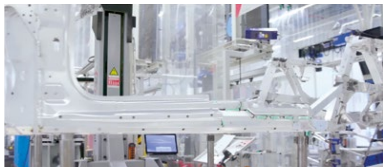
Display of welds on the body with one of the six laser projection systems in the background.
