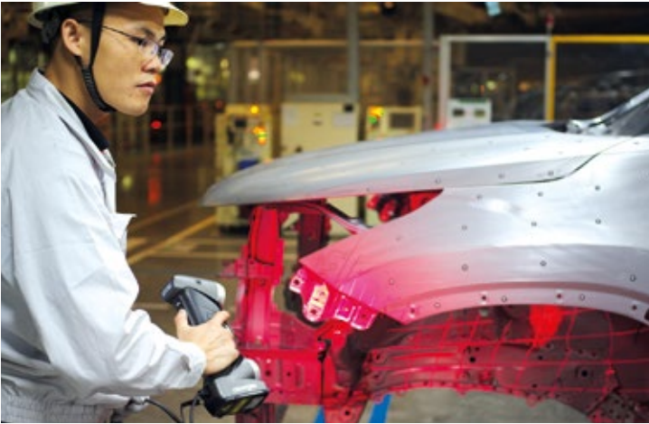
Flexible quality control: Combined scanning and probing for the shape inspection of a car rim
