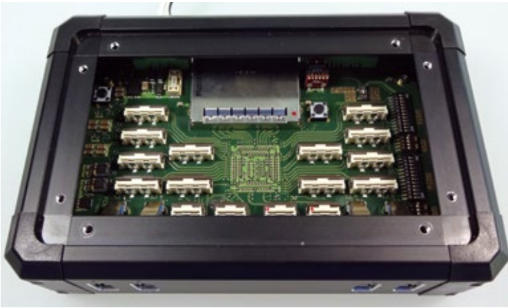
The Ximea xSwitch offers up to 24 PCIe camera ports, up to 8 USB3 connectors, synchronization, and a bandwidth up to 64 Gbit/s.
