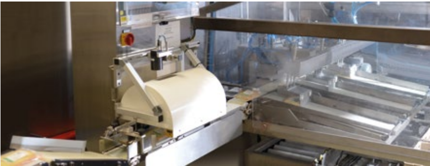
The cheese packaging passes under the machine vision system from the left and is placed in transportation boxes after inspection.
