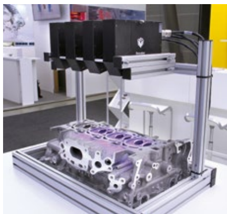
Gocator Volume Checker inspecting engine cylinder heads.
