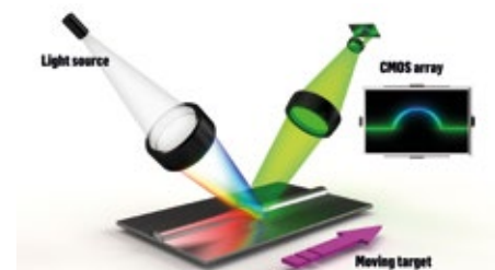
Fig. 2: Line confocal imaging principle.
