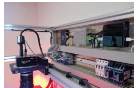
Programmable external frame grabber (center) and Intel NUC Mini PC (right)
