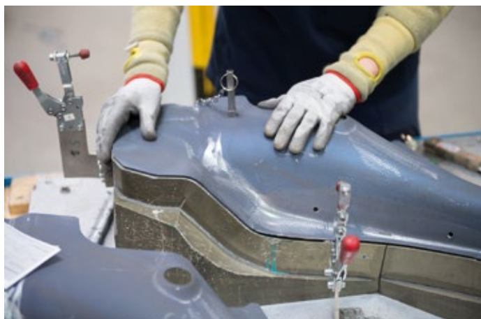
The hot stamped parts are given their final form in the laser cells. After machining, the employees perform random sampling to ensure fitting accuracy.
