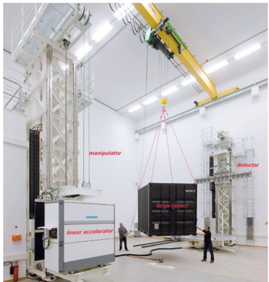
► Fig. 4: Interior of the high energy test facility. The radiation source and detector can travel at height by means of a tower system, in order to scan large objects and generate projection images of up to 4.6 \times 4 m (height x width) with a 400 \mu\text{m} sampling distance.
