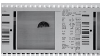
Typical film image from Surveyor mission with a CRT display (left) and associated data fields (right)
