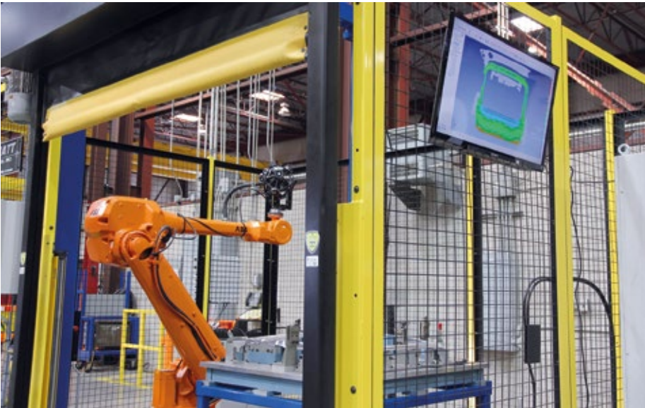
An automated quality control solution using optical reflectors to carry out accurate and repeatable measurements on the shop floor.
