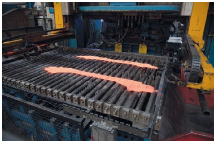
The parts are heated to 950 degrees and placed in a press to shape them.
