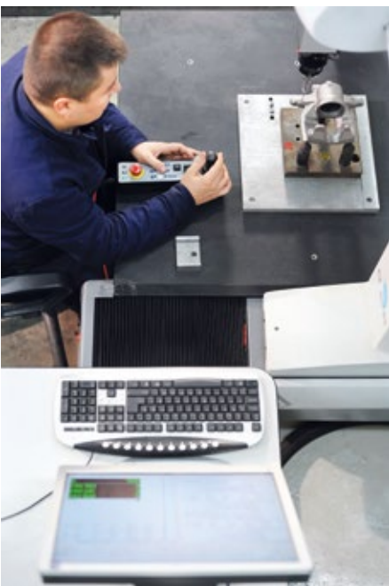
Metrology inspection carried out on traditional equipment in the measuring room.
