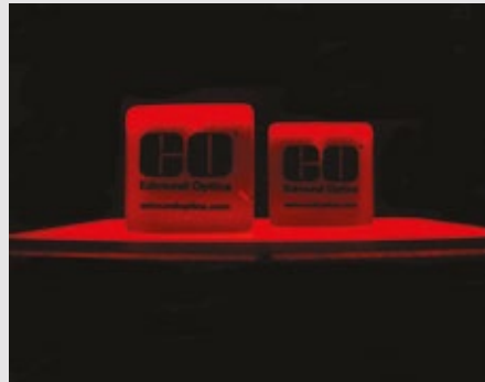
Image taken with fixed focal length lens (entocentric lens)
