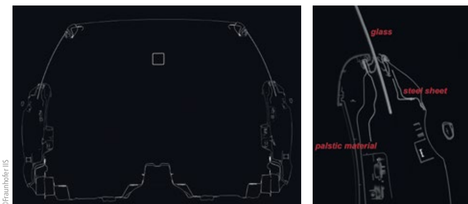
Fig. 6: CT sectional image through the passenger safety cell (left) and enlarged image of the door area (right).
