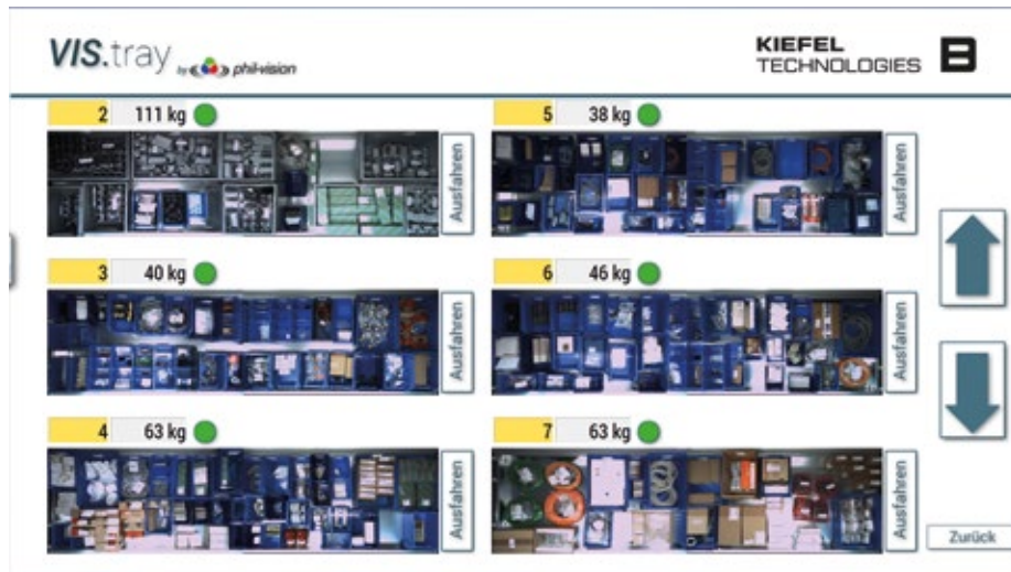
By scrolling the operator can find out quickly which trays still have space and weight capacity for the storage of further parts.
