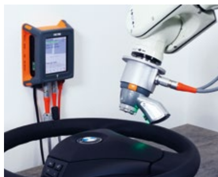
Fully automated solution: Profile measurement integrated with robot.
