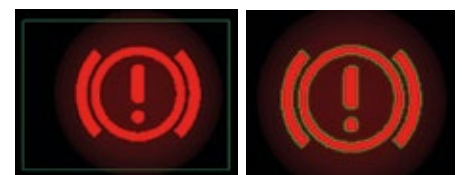
Comparison of static POI manually drawn in the software and Auto-POI (Automatic Points of Interest) adapted to an object based on color tolerances
