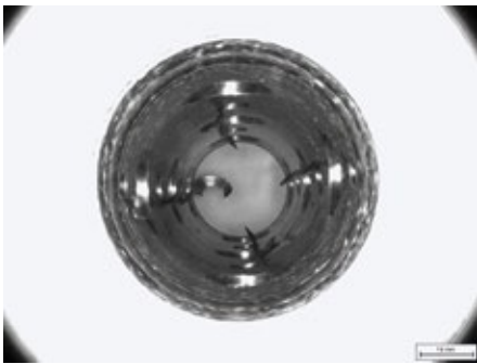
Bore hole inspection of cross bores (diameter 15mm, depth 40mm) with chip remains from the drilling process
