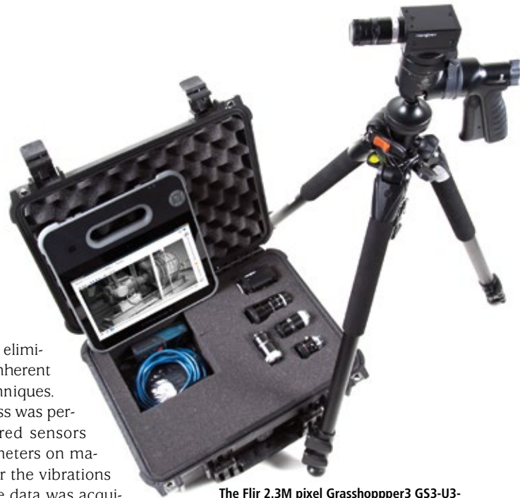
The Flir 2.3M pixel Grasshopper3 GS3-U3-23S6M-C camera, which is mounted on a Vanguard tripod, acquires monochrome image data at a default resolution of 1,920 x 1,050 and at a speed of 120 frames/sec.
