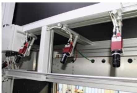
5 Megapixel Manta G-504 for the attributive inspection and color recognition
