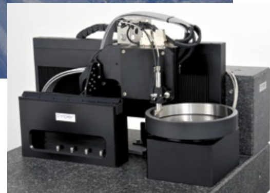
The device CT R200 with white-light sensor on top of a massive granite platform
