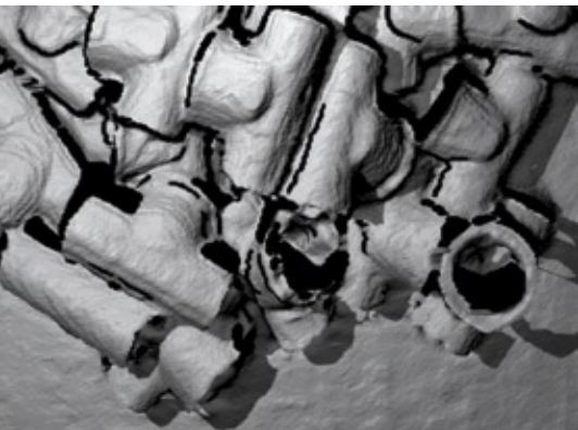
A typical 3D point cloud acquired with a laser scanner. The cloud shows clutter in form of a background plane, missing data, and occlusions.
