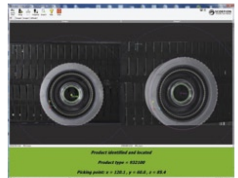
A screen shot from Scorpion Vision's 3D camera as it takes a picture of the wheels
