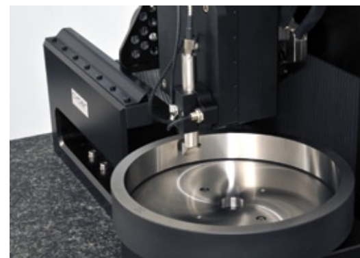
The surface of a round part is inspected for defects
