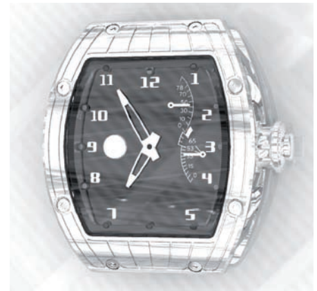
Application Example: Raw image result of the glass window of a watch as seen by a vision system
