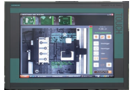
The user interface of the Simavis P image processing software on the Simatic flat panel monitor Pro specifies whether the test criteria have been fulfilled
