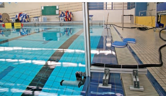
▲ Starting and turning overview: the start, the diving phase and the first underwater phase are recorded synchronously by one camera underwater and one above the surface. Further phases are monitored by single cameras.
