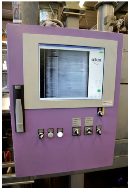
Optical final inspection by the Octum CV-600 system
