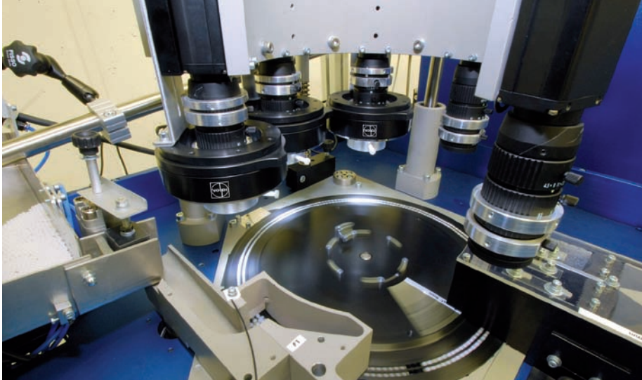
Automatic inspection system for surface and dimensional inspection of glass, plastic and metal spheres; camera systems inspect the entire sphere surface
