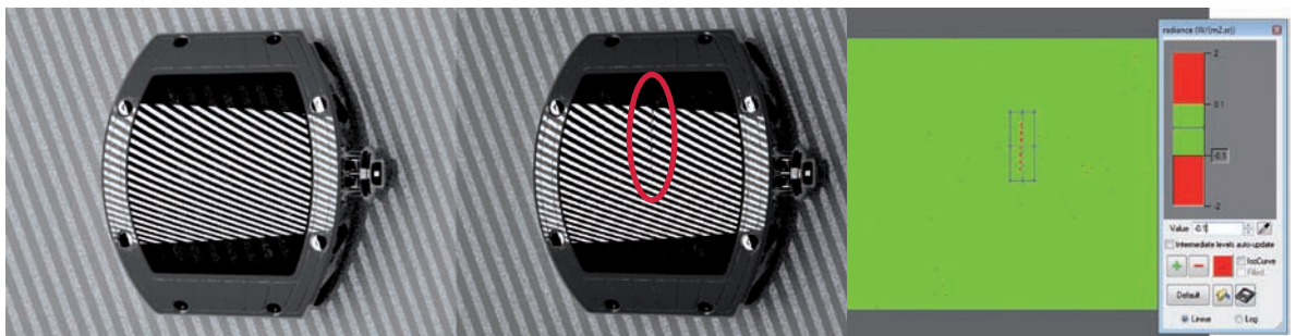
Virtual defect detection in the result simulation of the subtraction of two camera images
