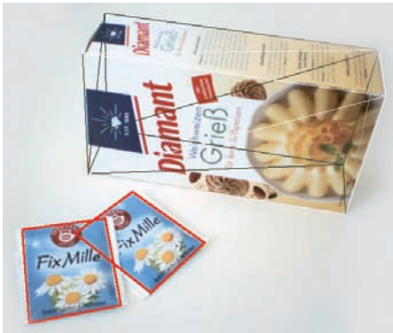
Fig. 2: Recognition and localization of different objects. For 3D objects, the 6-DoF pose is computed with the Keyetech 3D Extension.
