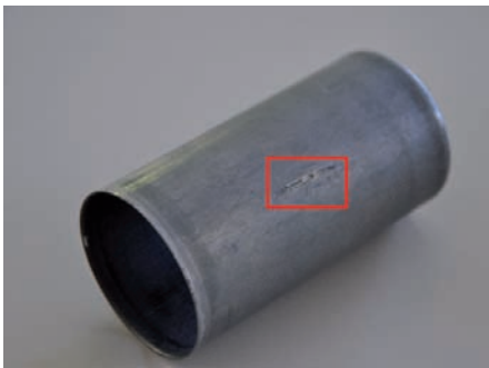
Finished tube with defects
