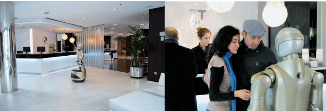
With its integrated touch screen, the service robot REEM-H provides information to the guests of a hotel, e.g. the weather forecast or the sightseeing hot spots
