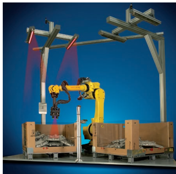
Fanuc’s M710iC 50 stereo-based Bin Picking system has integrated vision into their robot controller
