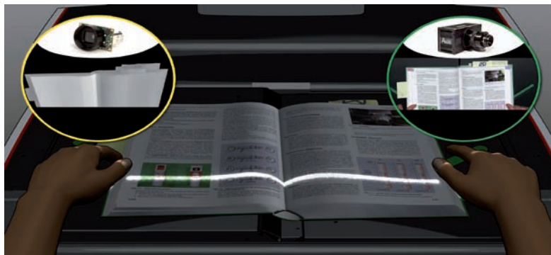
The line scan's projection is moved over the book (green) while the area scan camera (yellow) is pointing down at the cradle
