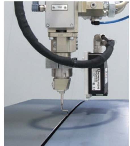
A special hook application nozzle ensures seam sealing directly at the door gap
