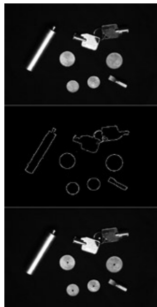
Fig. 4: Grey-level image (top), edge image (centre) and result of the Hough-transform for circles (bottom); points are depicted as overlay with the original image to show the centers of the circles detected. Mind the white point as centre of the partly occluded metal ring.
