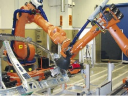
InfraTec's automated thermographic testing system for non-destructive testing of body panels in the automotive industry
