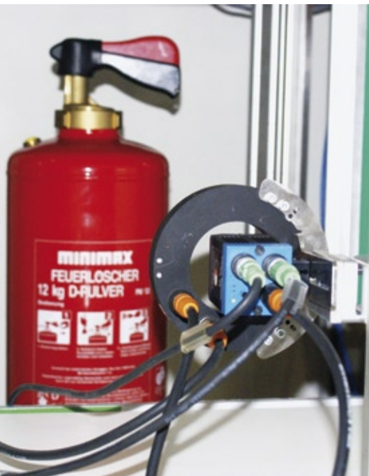
The Eyesight Advanced Vision System by SensoPart identifies fire extinguisher containers based on different geometry and colour characteristics. An LED ringlight ensures optimal illumination
