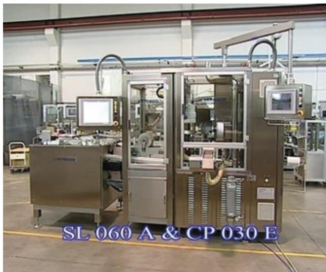
Face-powder compacting machine, complete with robotised loader and machine vision system (Courtesy of Vetraco Group)
