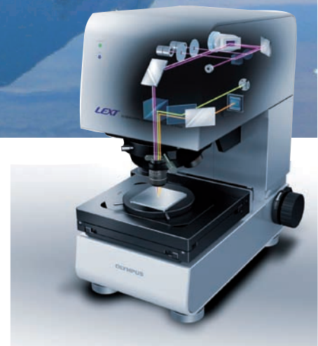
Schematic of the laser and brightfield light paths of the Lext OLS4000
