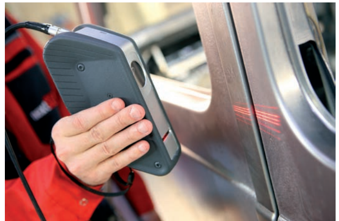
The tilt angle between device and surface is recognized and used to correct each measurement so that the final result is a true normal section, independent of the sensor's alignment
