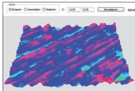
Fig. 4: Roughness and principal orientation of a mached wood surface can be determined easily with shape-from-shading methods.
