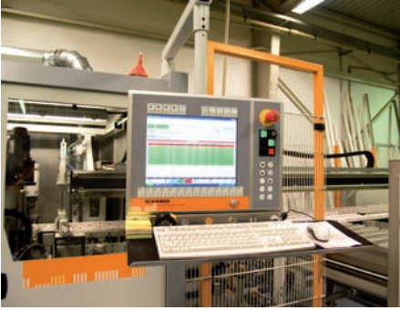
The operator can always see the current production process with the graphical user interface VisionView
