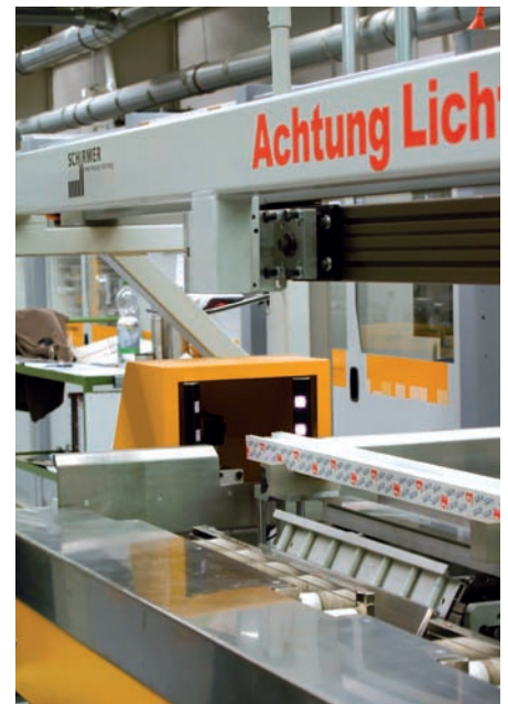
The In-Sight Micro 1100 from Cognex checks whether the rectangular tubular window frame put on by hand matches the IT system specification
