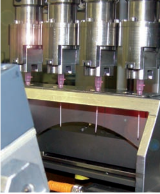
The completed infusion sets are checked with respect to 100% quality and completeness
