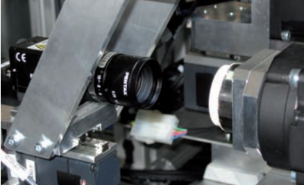
The defect detection is performed with an accuracy down to 10 µm
