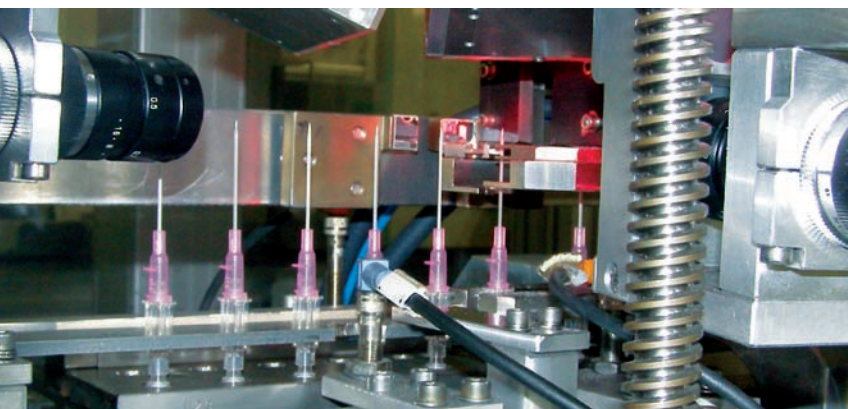
Vinspec checks the needle point in the \mu\text{m} -range
