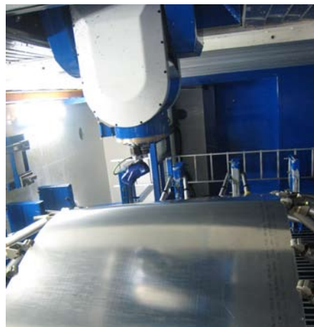
Zephyr is scanning a part of the Airbus A380
