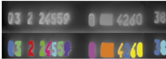
The 3D raw data with height data coded as grey image at the top and at the bottom, the segmented characters
