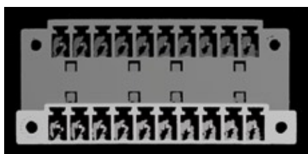
Height profile of the specimen: darker areas are farther away from the camera
