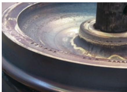
The stamped characters on the railway wheels are used for traceability
