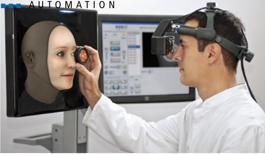
Using a head-mounted display and a model head, physicians can train retinal examination procedures in the same way as with a real ophthalmoscope
