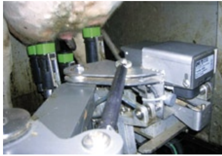
The TOF sensor is small in size and low in weight, allowing it to be easily mounted on the robot arm
