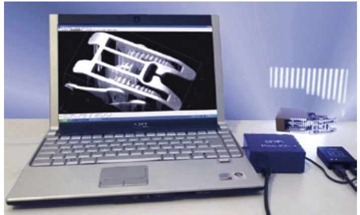
Pico DevKit with pico projector, a development platform for the digital light projection
