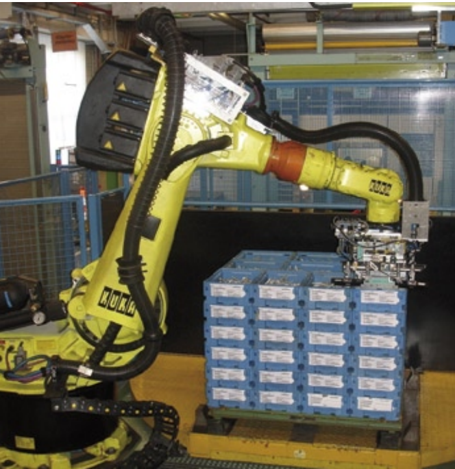
A robot depalletizes small load carriers automatically
