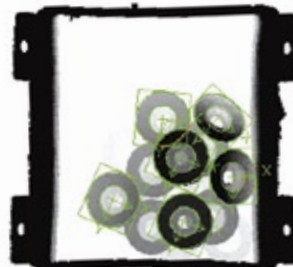
The software recognizes the position of the brake disks
