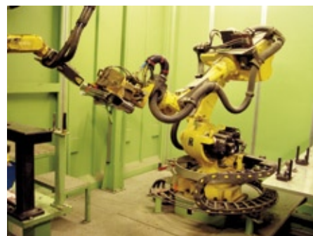
3D welding seam inspection is the basis for process optimization and automated repair (Image: Vitronic)
