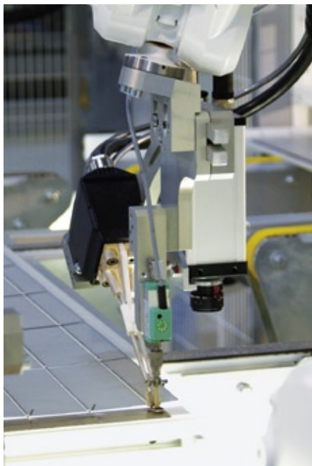
Robots deposit the foils and soldering ribbons and position the soldering points accurately, based on the part position location
