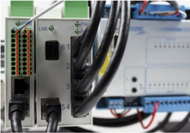
The trigger device is assembled on DIN rails
