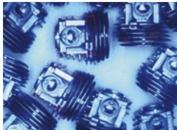
A machine vision system detects position and orientation of cylinder heads for the automatic loading and unloading of machining centers
