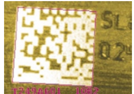
Fig. 4: The data code reader reads defocused as well as damaged data codes, even if the whole finder pattern is missing.
