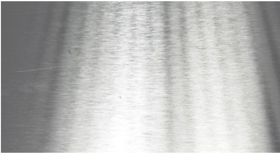
Picture of a metal strip. The light/dark transitions are called chatter marks
