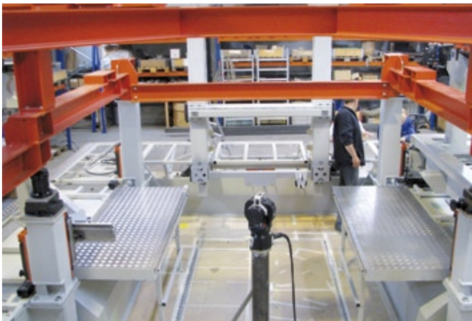
The Laser Tracker (middle of the picture) is used for measurement, justification and und positioning of the mount.
