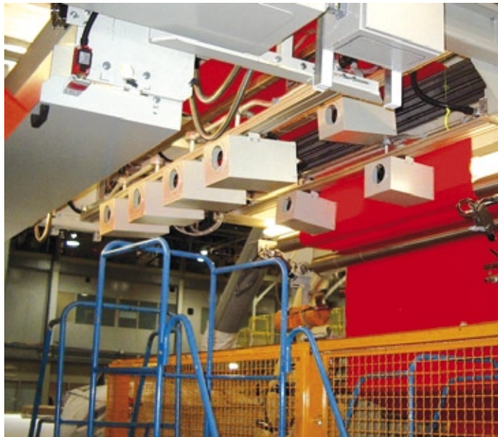
The position of a Shelton WebSpector system in a textile production process is not restricted as it is for manual inspection
