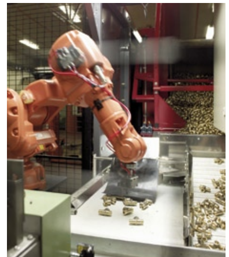
The parts are moved in single layer into the position underneath the camera by the tipper and the loop of the Multiflex compact feed system
