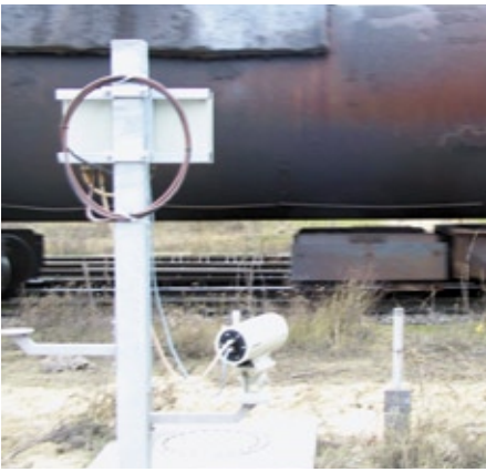
Torpedo cars carry large amounts of molten iron to the converting plant for final processing. Two infrared cameras monitor the condition of the refractory lining in the cars
