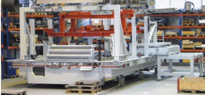
Assembly mount for the Airbus – exterior and interior. In red: Simulation weight for the later fuselage.
