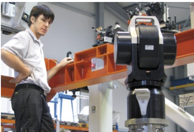
Special holes within the construction, which simulates the weight of the fuselage, enables measuring the lightweight construction taking realistic production preconditions as a basis.
