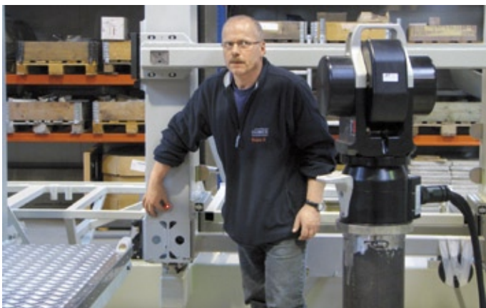
Measuring a reference point at the assembly mount done by technician in measurement technology August Katteneder.
