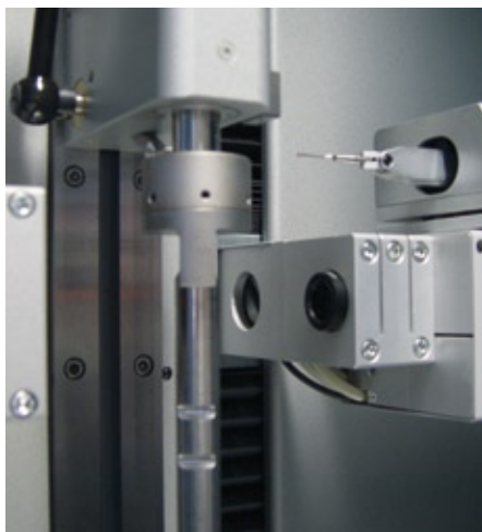
Non-tactile optical scanning of a work piece
