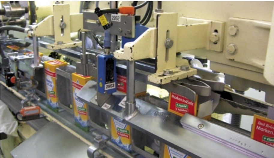
Sensor-monitored salt packaging plant
