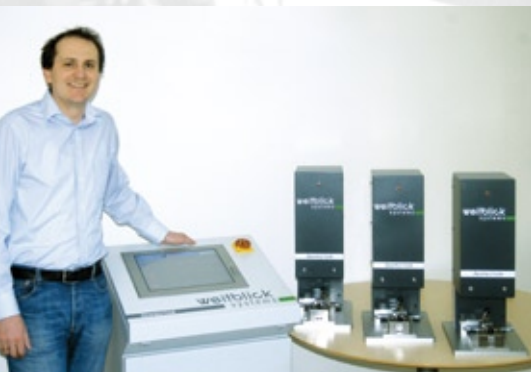
Rainer Reisinger, CEO weitblick systems, demonstrates the automatic measuring system which consists of three measuring stations and a controller with an integrated PC
