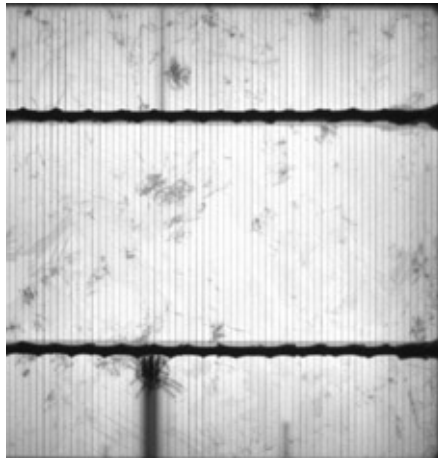
Finger electrode defects in the PV cells are clearly seen as darker regions indicating lower or lack of light emission. Image has been taken with Andor Luca R camera and composed from four accumulations each acquired for 8 s (image courtesy of Dr. Karsten Bothe, IFSH, Hameln, Germany)
