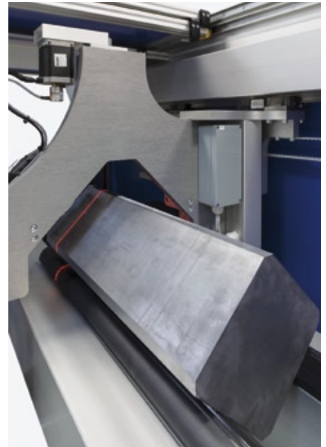
▶ Four laser scanners placed on the sensor base plate measure the master part
