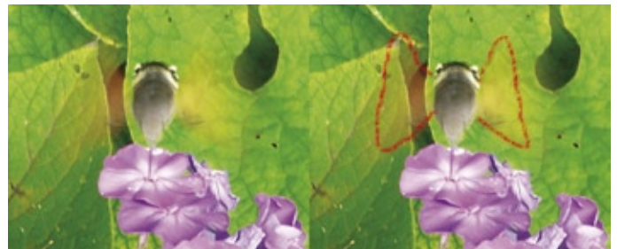
Fig. 2: Smear in an image captured by a progressive scan camera, to be seen in the region of the fast moving wings of the Hummingbird-moth; integration-time: 25 ms.
