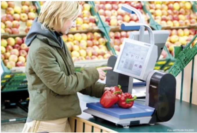
▲ The compact USB camera auto-detects the products on the scale
