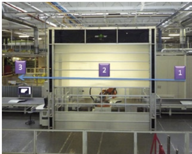
Fig. 2: Examining sequence. 1: Feeding parts onto entry conveyor belt, 2: Inspection cell with ABIS II, 3: Exit conveyor belt with indication of inspection results
