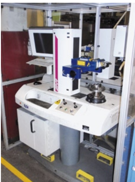
General view of the precision measurement machine for semi-automatic measurement of synchronizer rings
