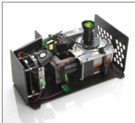
The fully functional integrated Luxbeam DLP Light Engine modules include the pre-installed software and the light source as well as all electronic and optical components
