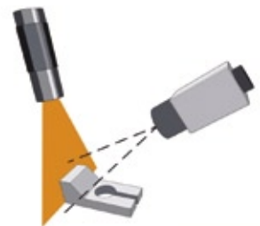
The 3D shape of an object is determined by measuring the profile of the object along a projected line of light.
