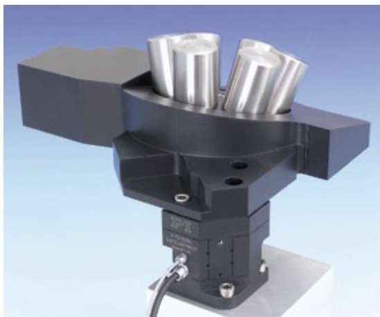
Fig. 2: Piezo drives can be flexibly and easily mounted on a microscope to allow rapid fine tuning of the focus. It is thus possible to travel several hundred microns in only a few microseconds and with an accuracy of a few nanometers (Photo: PI)
