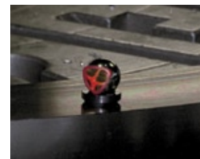
Measuring directly on the turning mill: Michael Gerards, Precision Mechanics Foreman, checks about 30 points on the casting using a reflector
