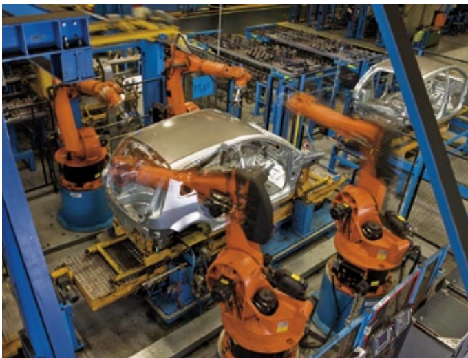
The path to more quality: Fully automated gauging cell for inspecting even the hardest to reach measuring points
