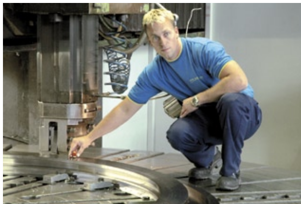
Measuring directly on the turning mill: Michael Gerards, Precision Mechanics Foreman, checks about 30 points on the casting using a reflector
