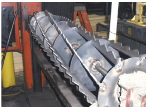
Fig. 3: On a farm tiller welded component, a total of about 60 welds per part having an average length of 35 mm, are done in a robotic gas metal arc welding cell
