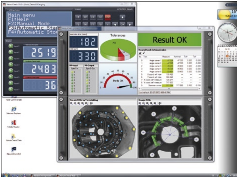
Shop floor (automatic) operation in NeuroCheck 6.0 featuring Control Panel (back) and Process View (front)
