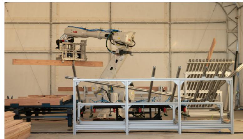
[ABB and Cosmic Buildings](#) are using AI-powered robots to make rebuilding in Southern California more efficient. The combination of ABB's IRB 6710 industrial robot, digital twin software, and Cosmic's AI-driven Building Information Model (BIM) optimizes the construction process.
