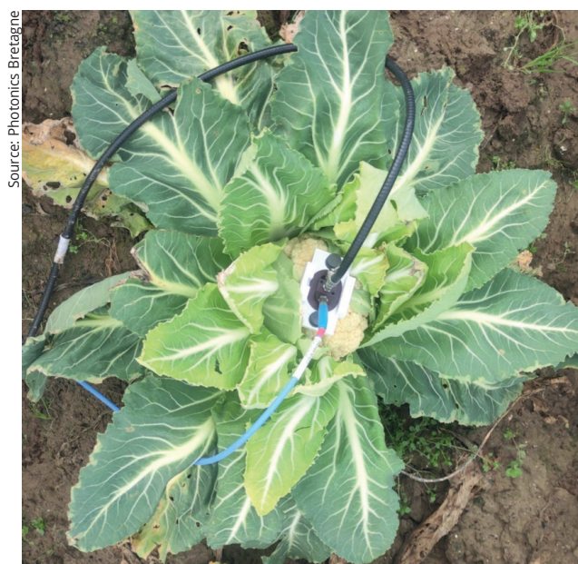
Probing the nitrogen amount in cauliflower using a reflectance signal developed by Photonics Bretagne
