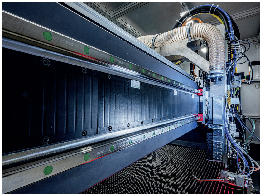
Hiwin supplies linear guideways and linear motors for the construction of the 10-ton portal machine
