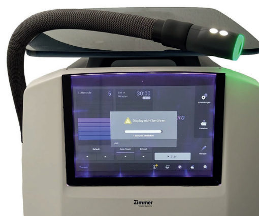
Fig. 5 Self-disinfecting touchscreen fitted to the Cryo7 cryotherapy device from Zimmer Medizinsysteme during disinfection. The visible violet impression is not caused by the UVC LEDs but by additional violet LEDs (modified as per [3])
