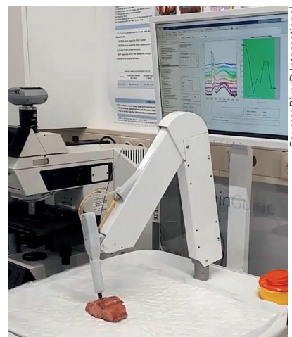
Fig. 3 Raman system to assess soft tissue resection margins
