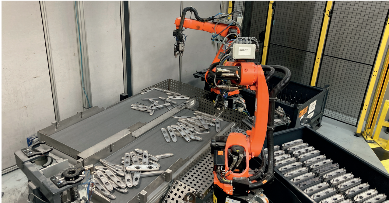
Robots pick components from a box at the Cikautxo company that are lying in a disorderly fashion and then place them in a specific alignment.
