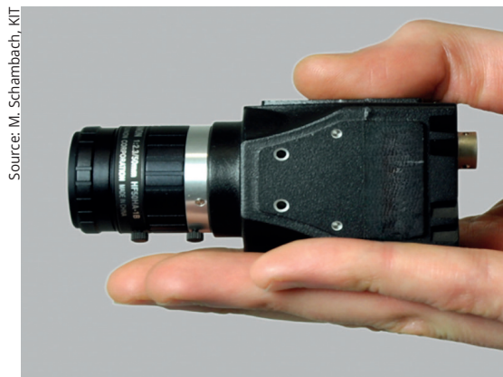
A multispectral version of a light field camera
