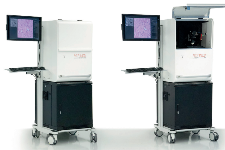
Fig. 5 Refined Laser Systems' intraoperative microscope prototype for the identification of tumor margins in the surgery room (Source: Refined Laser Systems)
