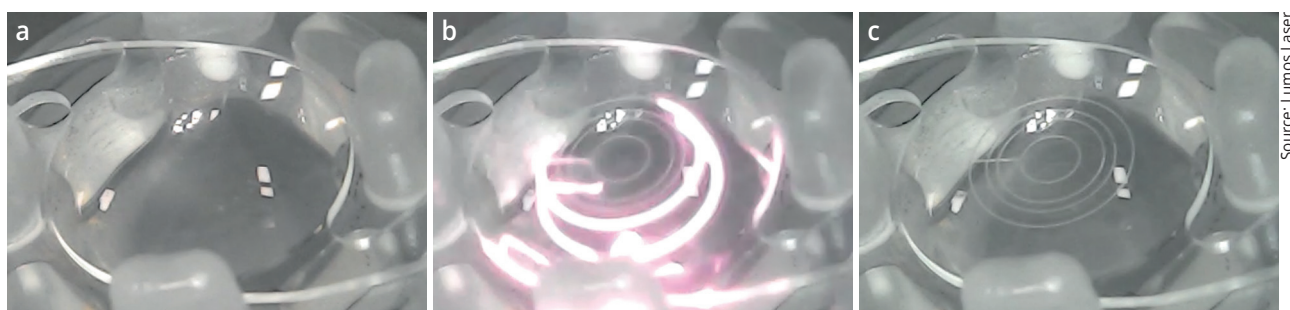
Laser cutting of an IOL lens: (a) before; (b) during; and (c) after the laser process
