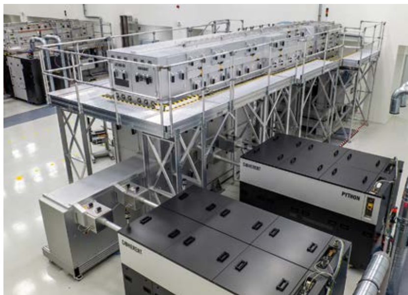
Fig. 2 LineBeam 1300-G8 with TwinPython laser to anneal GEN 8.7 mother glass. The TwinPython delivers four beams at 355 nm and 600 Hz of 1 J each to the LineBeam system (Source: Coherent)
