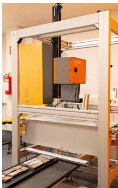
The Specim FX120 LWIR hyperspectral camera mounted on the 100 x 50 Lab Scanner in the Specim demo lab measuring mineral samples. (Source: Specim)
