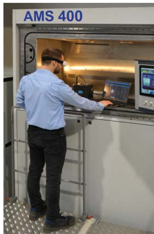
Fig. 3 Before starting the measurements latest parameters are checked by the engineer and the system is adjusted by using the pilot laser
