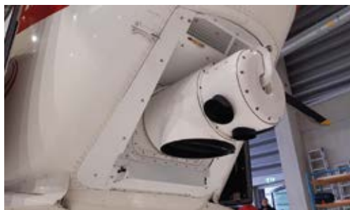
As part of the BMBF-funded project “CHARM – CH 4 Airborne Remote Monitoring”, the Adlares helicopter (top right) with a lidar system on board (right) flies at a speed of 300 km/h along a gas pipeline several 10,000 km long to detect gas leaks (left)
