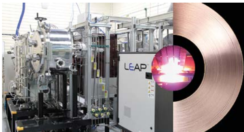
Fig. 6 PLD manufacturing of HTS tapes (Source: Coherent / Faraday Factory Japan)
