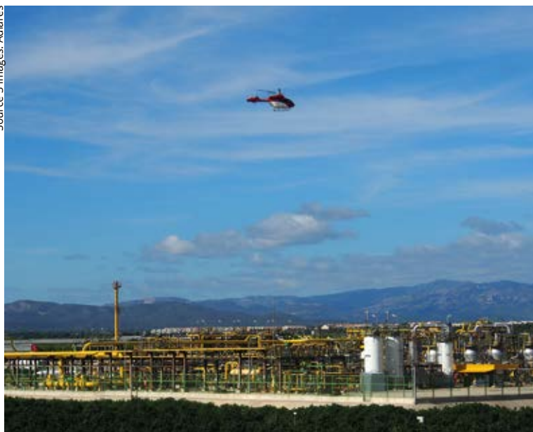
As part of the BMBF-funded project “CHARM – CH 4 Airborne Remote Monitoring”, the Adlares helicopter (top right) with a lidar system on board (right) flies at a speed of 300 km/h along a gas pipeline several 10,000 km long to detect gas leaks (left)
