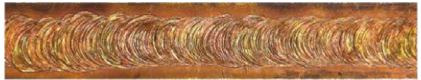
Fig. 5 Weld seam of 3 m/min 8 kW copper welding
