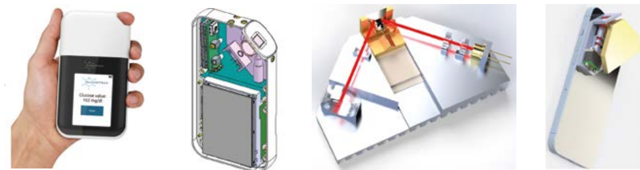
Fig. 5 Diamontech's handheld D-Pocket glucometer (under development); from left to right: top view of display and measuring site on the upper left side; cutaway view of optics and electronics; schematic display of QCL excitation and photothermal detection, and display of the complete optical unit on a smartphone for size comparison
