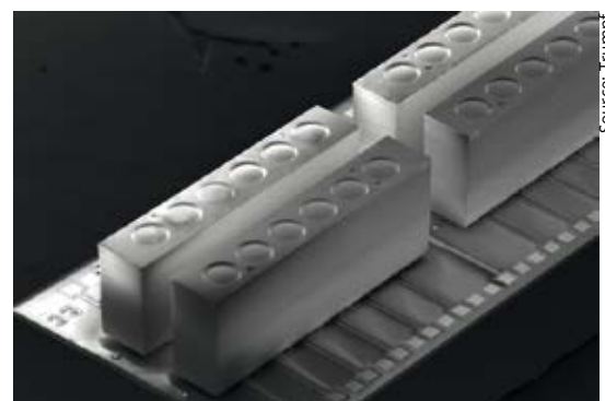
Fig. 3 SEM picture of 1 \times 6 bottom-emitting VCSEL arrays with integrated collimating lenses. The VCSELs are mounted on a carrier for characterization.
