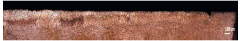
Fig. 6 Longitudinal macrograph of 8 kW and 25 m/min copper welding
