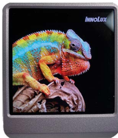
2.56-inch 4K VR LCD single-piece display demonstration (Source: Y.-H. Wu et al.)
