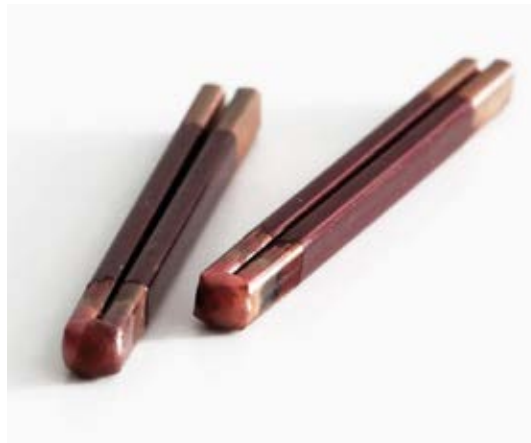
Fig. 9 Hairpins welded with an MPLC-based system
