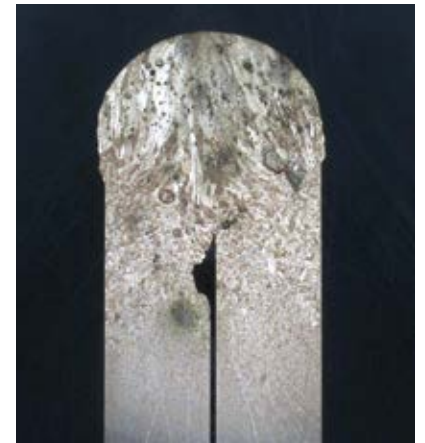
Fig. 10 Macroscopic of the hairpins welded with an MPLC-based system
