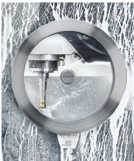
The principle of the rotating viewing window, originally from the maritime industry, allows an outside view of the processes inside the machine. The Rotoclean C2 lens uses the same principle: It has a fast-rotating viewing window made of shatterproof glass.
