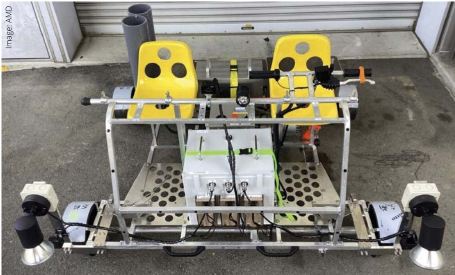
At the heart of the track inspection solution is a vision computing box attached to a cart that inspects tracks at speeds of 12 mph. The box features a high-speed camera that uses the FPGA-based Kria K26 SOM for AI-enhanced pre-and-post data and image processing.
