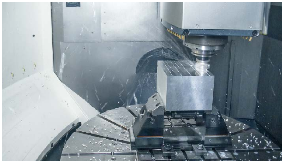
Flying metal chips not only obstruct the view of the tool and workpiece but also become dangerous projectiles that can cause significant damage inside the machine.
