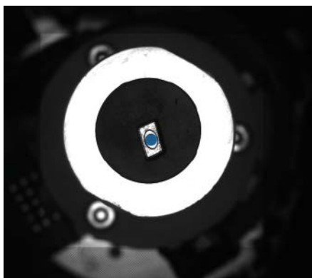
Detection of the component center from below for position correction before placement on the pin pallet
