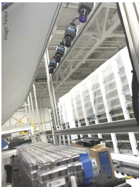
AI improves inspection performance and is used to identify rust. Tensor ID uses four high-resolution cameras from Teledyne Dalsa to inspect the battery module.
