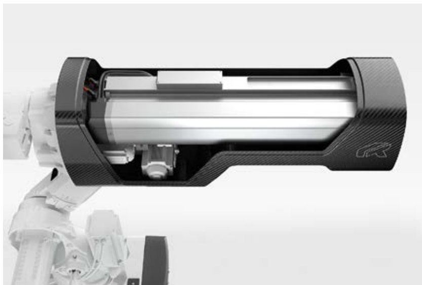
Luxinar SR laser integrated with a robot for automotive production (Source: Robot Technology)
