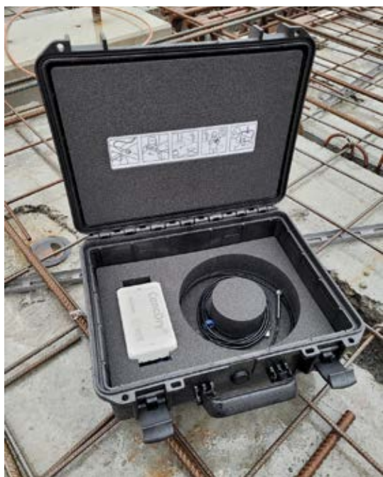
ConcDry in its right element: a humidity and temperature sensor system made to monitor concrete drying, based on Shute's patented polymer optical fiber sensor technology.
