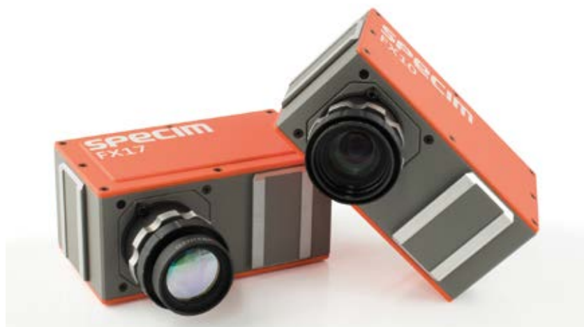
Fig. 3 Specim's FX10 and FX17 hyperspectral cameras are the key components for the fruit inspection system, covering a wavelength range from 400 to 1700 nm. (Source: Specim)
