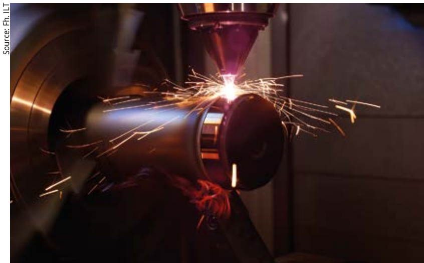
The SMaC process: coating with EHLA and time-parallel mechanical machining. The coating is several hundred degrees hot immediately after being deposited and therefore has only a fraction of its regular hardness.
