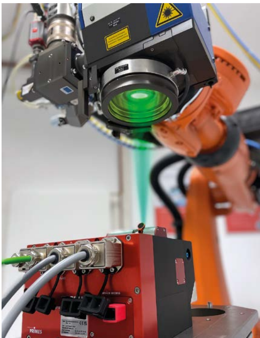
The FocusParameterMonitor (FPM) monitors the relevant laser beam properties during production. (Source: Primes)
