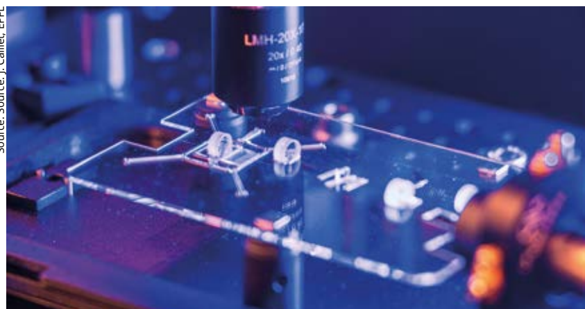
Scientists from EPFL's Galatea Laboratory make gigafemto lasers on a glass substrate.
