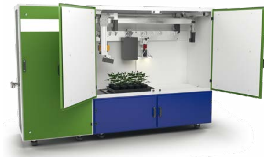
A semi-automated phenotyping system for laboratory samples that enables measurements with a range of optical sensors, including hyperspectral cameras, chlorophyll fluorescence cameras, RGB cameras or laser scanners. (Source: Nynomic group)
