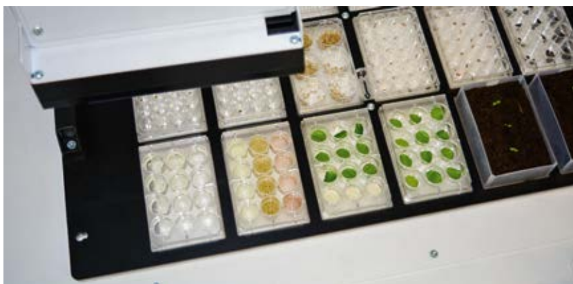
Phenotyping is the quantitative recording of plant appearance. Environmental influences or the effects of plant diseases are identified using optical methods. For this purpose, leaf discs are grown in multiwell plates and analyzed using dedicated camera systems. (Source: Nynomic group)
