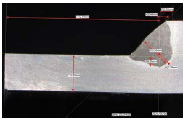
Fig. 4 In a research project conducted at the Scansonic laser laboratory, different parameters are varied in order to develop an optimal welding method. This project showed that results could be achieved with a disk laser that were comparable to those achieved at WMG with a ring spot laser. In this example: 3 mm material thickness, AL6082 aluminum, and 5 m/min process speed at 7.5 kW, oscillation 180 Hz, amplitude 0.8 mm, and spot diameter = 0.7 mm. (Source: Scansonic)
