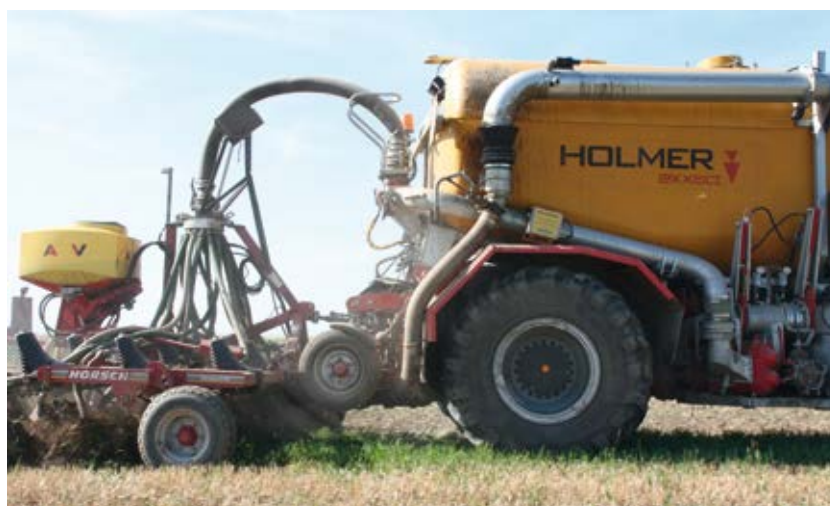
In this application an NIR sensor is directly mounted on the slurry tank, measuring the nutrient concentrations of organic fertilizer. (Source: Nynomic group)
