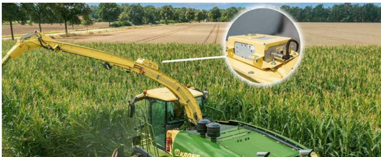
An NIR sensor directly mounted on an agricultural machine is shown in operation. The use of this technology allows not only dry matter, but also starch, sugar, or many other quality parameters to be determined, depending on the crop. (Source: Nynomic group)
