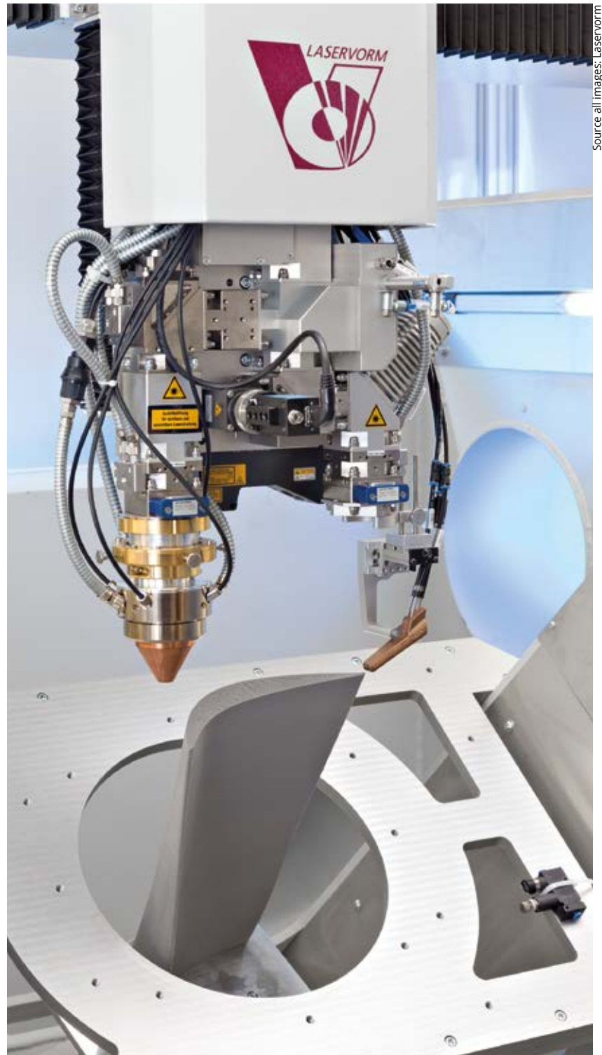
Fig.1 Tracing of the parameters is important for safety-relevant applications like turbine blade repair to control the cladding process.
