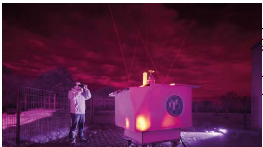
Fig. 6 The mobile lidar system sends five beams into the night sky. With four small and one large telescope, it detects the photons from up to 100 km altitude and provides climate data in real time.
