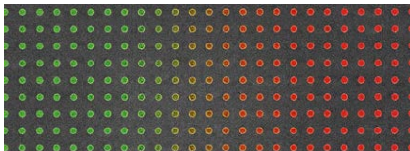
The new sensor consists of many metal nanoparticles that work together to detect hydrogen in their surroundings. (Source: Y. Strandqvist, Chalmers U.)
