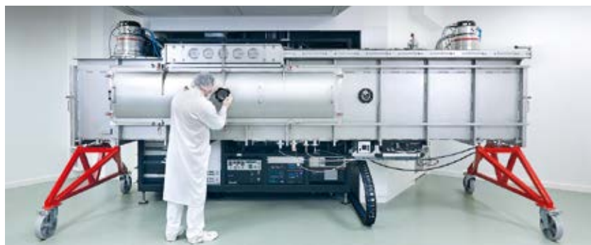
"Maxima", the patented IBS coating machine for large optics (long shapes)
