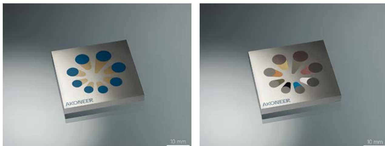
Fig. 6 Stainless steel sample coloring of Ekspla logo using FemtoLux 30 with GHz burst feature.
