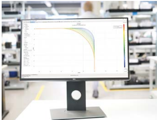
Fig. 3 The SCANmotionControl software displays various pre-calculated laser beam paths on the material for increasing velocities as a heatmap. Source: Scanlab
