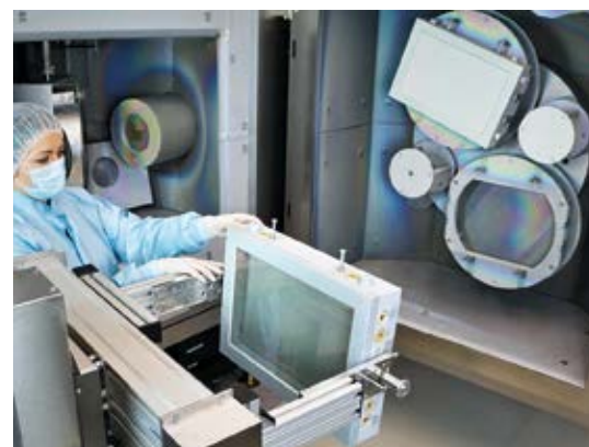
"Teresa", the largest IBS machine suitable for substrates up to \varnothing 550 mm
