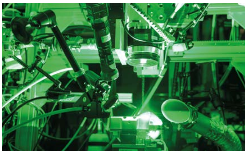
Trumpf and the Fraunhofer ILT investigated the laser welding of copper connections by using a particle accelerator (Source: Trumpf)
