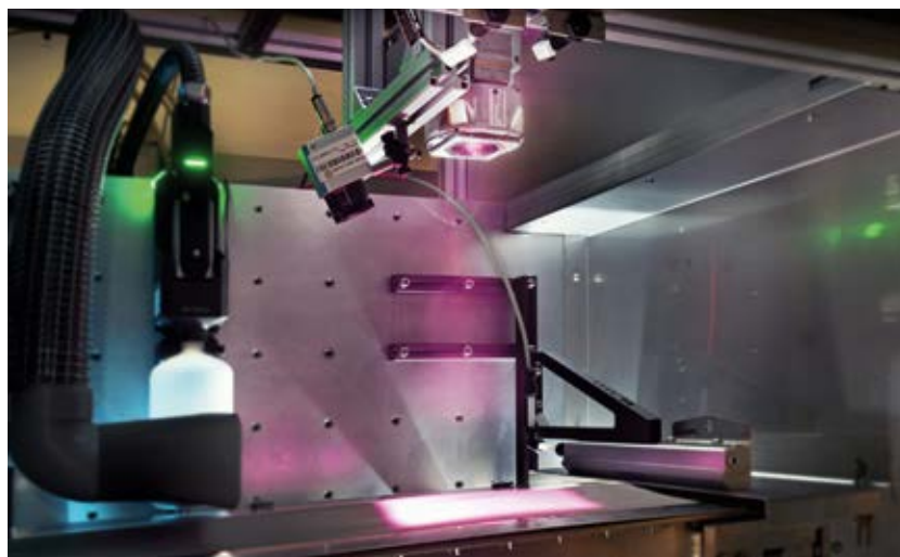
Laser drying system with large-area irradiation of the electrode (Source: Fh. ILT)
