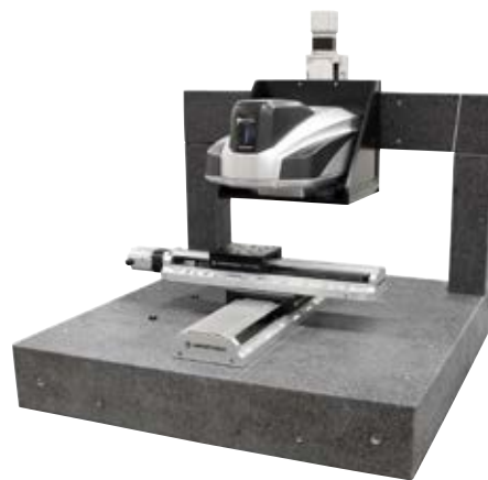
Integration of a Keyence VR5000 in an Aerotech positioning systems for even larger travel distances: up to 300 mm on a stable granite gantry.
