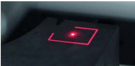
The red frame indicates the area to be laser-processed so that components can be precisely aligned.
