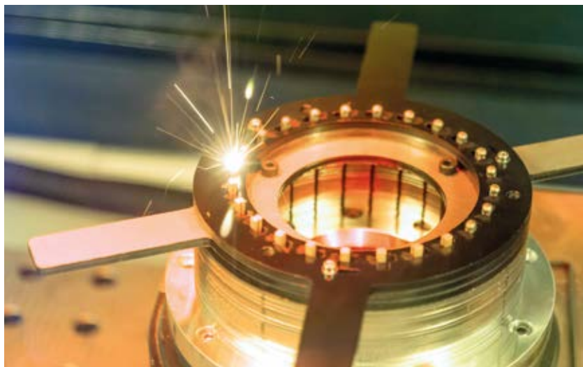
Welding hairpins: lasers for the manufacture of electric motors or e-car batteries are now an important business field for Trumpf.
