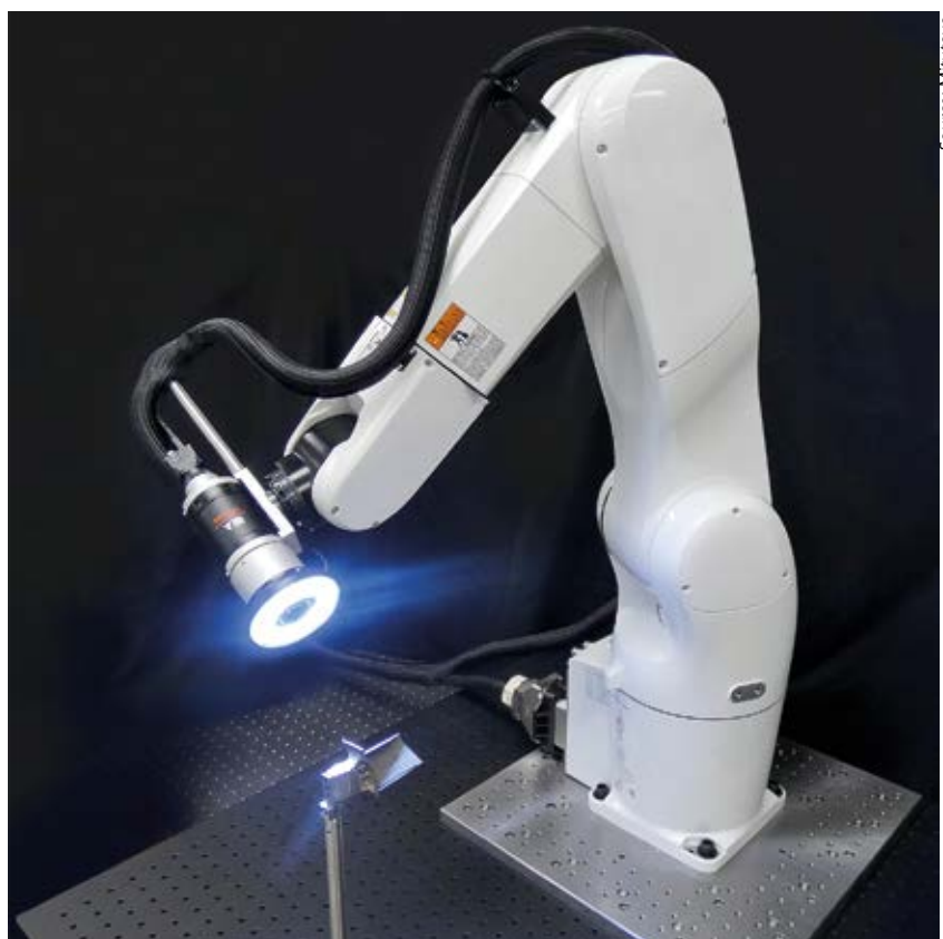
Fig. 2 New ROBOTAG system for high speed inline inspection and measurement
