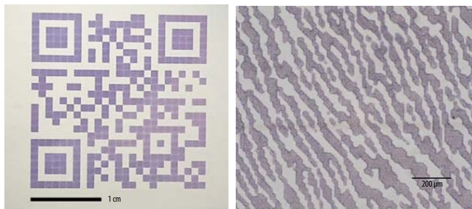
Fig. 5 Plasmonic marks made by laser implantation of gold nanoparticles: (a) QR-code, (b) Computer generated hologram
