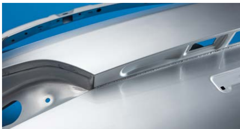
Diode lasers in the automotive industry: joining car body components
