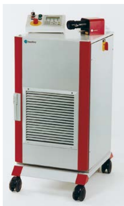
Early multikilowatt diode laser built in 1998 / 1999
