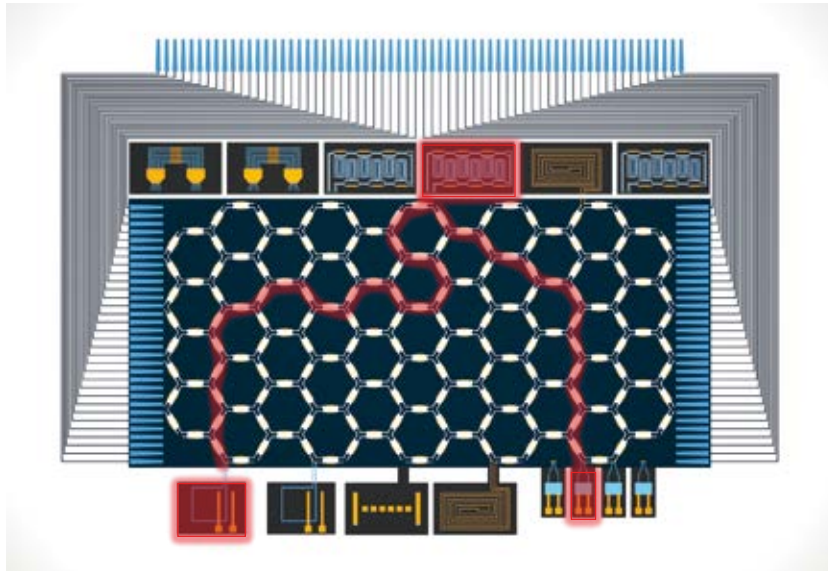
Fig. 2 Schematic representation of the programmable photonic device showing a more efficient delay line using a high-performance building block.
