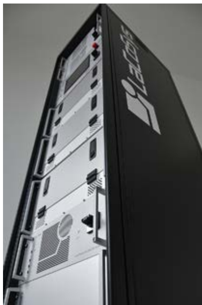
The new LaCoSys laser test system: the SmartPowerXL laser driver with a power range of 3,000 – 12,000 watts.
