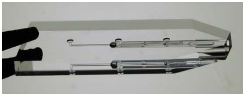
Fig. 5 3D microfluidic mixer for X-ray applications: determination of electronic structures during chemical reactions. (Source: Femtoprint, courtesy of SLAC)
